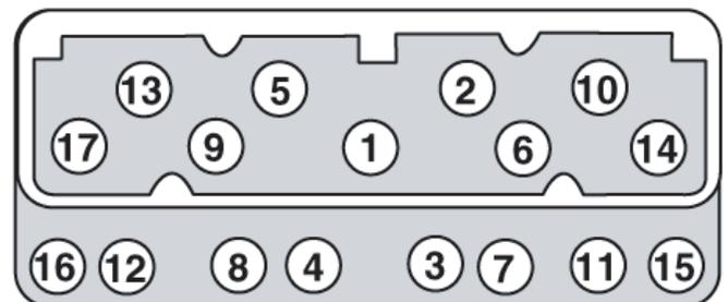
**Figure 3 - Cylinder Head Bolt Torque Sequence
