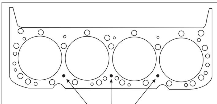
Drill three .125" holes in each head using 400 c.i.d. head gasket as a guide. **DRILL ONLY THE THREE LOWER STEAM HOLES** (closest to the spark plugs) as indicated. Drill straight into the head (90° from the deck) until the drill breaks through into the water jacket (about 9/16").
