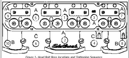
Figure 1- Head Bolt Boss locations and Tightening Sequence
