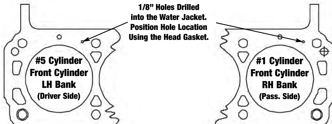
Figure 2 - Steam Hole Locations for Early 289 & 302 Engine Blocks
