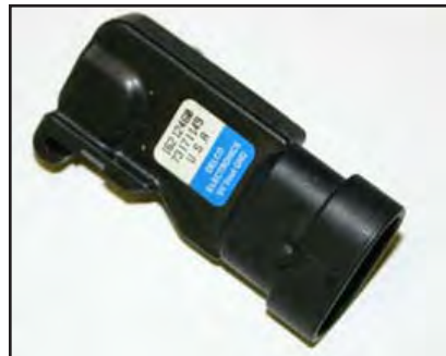
The Manifold Absolute Pressure sensor attaches to the harness with Connector J17.
