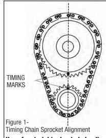
Use of a straight edge to help align the two timing marks is highly recommended
