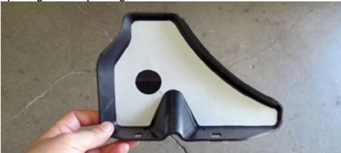
84. Install the water pump isolator onto the water pump bracket.
