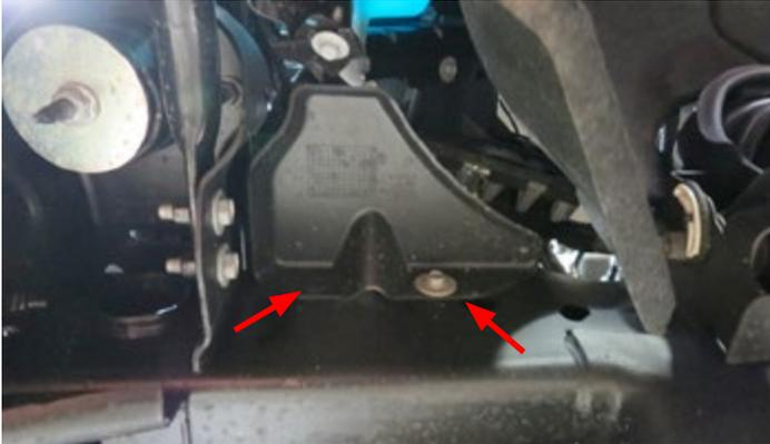
83. Cutout the supplied template and place it onto the splash guard. Using a drill with a 1.25" hole saw bit, drill out the opening in the splash guard.
