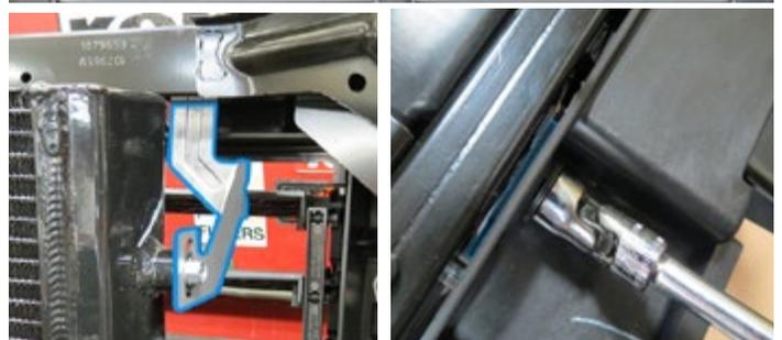
66. Using two (2) M6 x 16mm hex flange bolts from Bag #2, loosely secure the lower LTR brackets to the support brace where the push pins were removed from Step 60.
