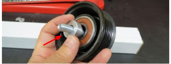
19. Using one (1) M10 washer and one (1) M10 x 40mm Hex Flange bolt from Bag #1, install the grooved idler pulley to the factory FEAD bracket. Torque bolt to 18 ft-lbs.
