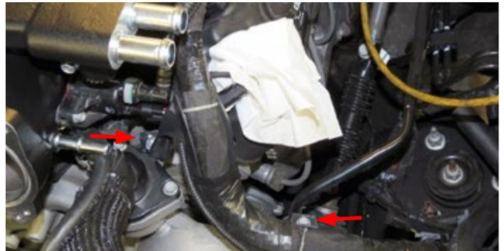
34. With the engine harness temporarily relocated, connect the factory EVAP hose to the EVAP solenoid.
