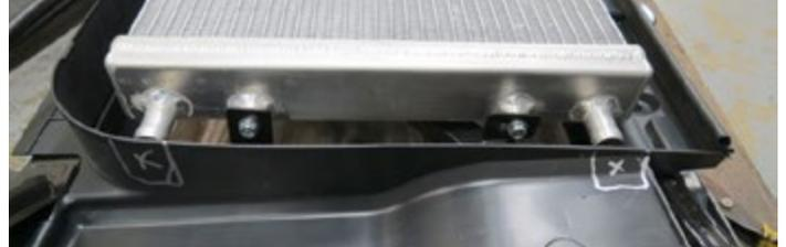
64. Trim the shroud using an appropriate cutting tool. Test fit the LTR hoses to verify proper shroud to hose clearance. Reinstall the weather guard and trim the rubber weather guard as needed. Re-secure shroud to support brace using the factory fasteners.
