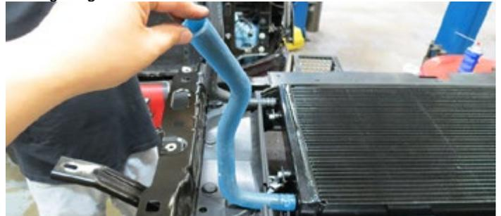
73. With the LTR secured to the support brace, carefully reposition the support brace by feeding the LTR hoses through the cavity between the radiator and the windshield washer fluid tank.
