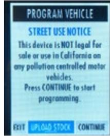
9. After selecting **SKIP** for the **CLOUD SYNC**, the **STREET USE NOTICE** will appear. Select **UPLOAD STOCK** and follow the prompts to complete the upload of the stock (.sul) file.
