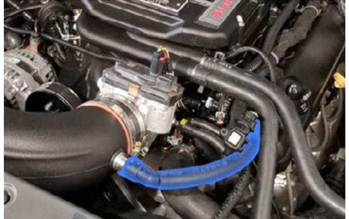
101. Fill the supercharger recovery tank with 50/50 coolant blend. See “How to prime the Edelbrock E-Force intercooler system guide at the end of these instructions.
