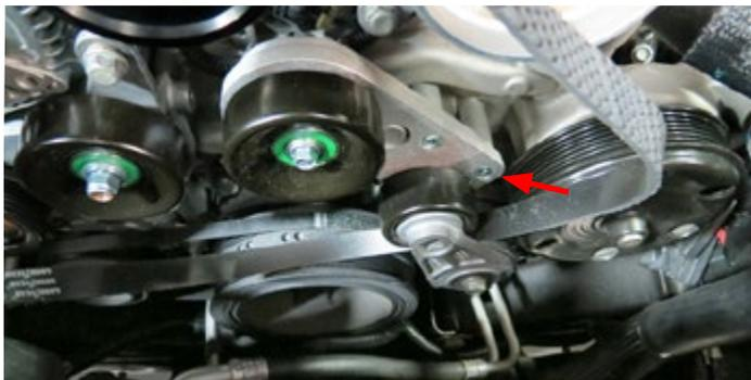
32. Using a breaker bar, rotate the tensioner counterclockwise and install the drive belt using the routing diagram below.
