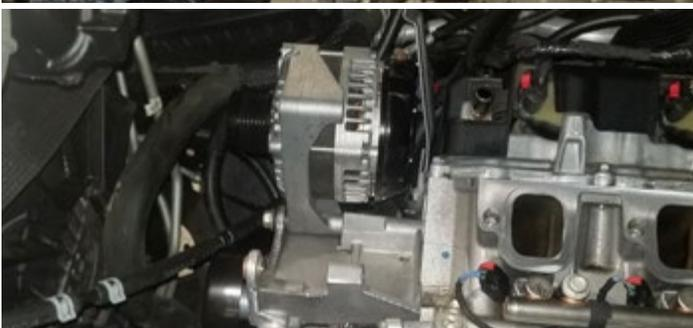
25. Remove the protective tape from the cylinder head. With the help from an assistant, carefully lower the supercharger into the vehicle. **(NOTE: Do not hold onto the bypass actuator when lowering the supercharger onto the engine).** Align the manifold to the engine before proceeding.
