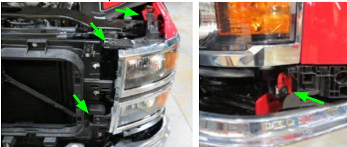
51. Carefully rotate the headlamp forward and disconnect the headlamp power connector. Repeat headlamp removal procedure for the passenger side headlamp.
