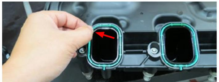
22. Clean and inspect the O-ring gaskets and replace torn or damage O-rings as needed. Using a razor blade, or equivalent, remove the tips off all eight (8) factory O-ring gaskets.
