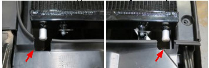
65. Using a 10mm socket, remove two (2) bolts securing the top of the shroud to the support brace. Position the upper SUV LTR brackets between the support brace and the shroud. Loosely secure them using the stock bolts.
