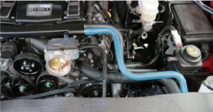
79. Using a 10mm socket and two (2) M6 x 10mm Hex Flange bolts from Bag #2, secure the recovery tank bracket to the recovery tank. Install the Recovery Tank to Water Pump hose to the side bars on the recovery tank and secure with a hose clamp from Bag #2.
