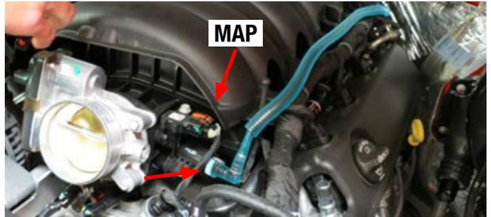
6. Detach the PCV hose located on the valley plate. On 5.3L applications the hose connects to the driver side of the intake manifold. On 6.2L applications, it connects to the front of the intake manifold.
