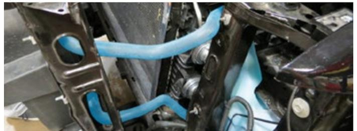
74. Re-secure the support brace to the chassis using the factory hardware.
