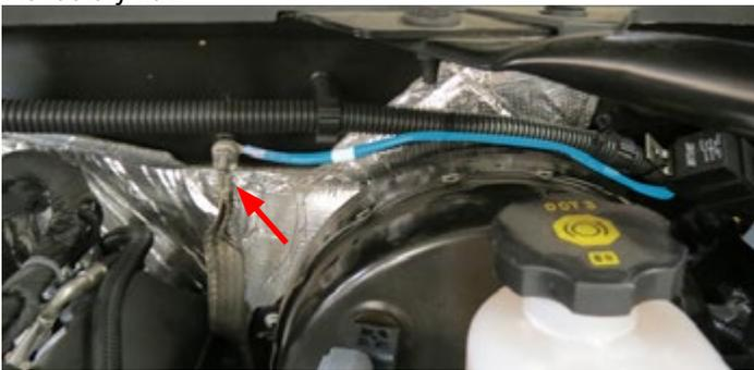
91. Route the POWER wire on the water pump harness to the power terminal located behind the fuse box. Using a 13mm socket, secure the POWER wire to the terminal.
