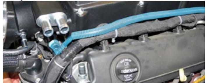
35. Install the straight fitting on the Valley to Nose PCV hose to the quick connect fitting located at the front of the valley plate. Connect the 90° end to the quick connect fitting on the manifold nose.
