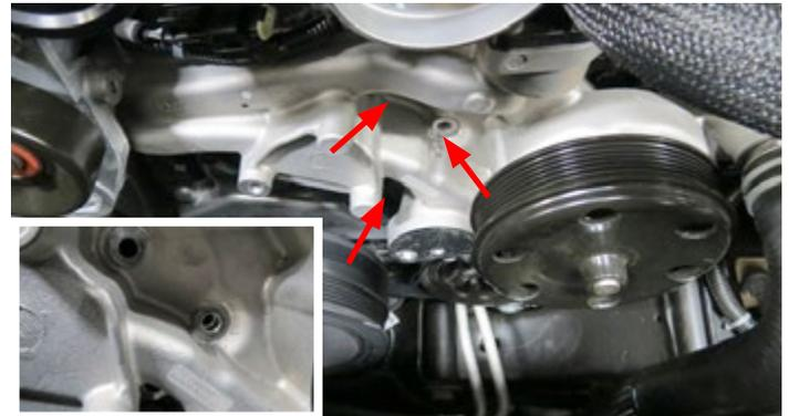
14. Using Blue thread locker and three (3) M8 x 130mm SHCS bolts from Bag #1, secure the FEAD bracket to the water pump using a 6mm Hex key. Torque bolts to 22 ft-lbs.
