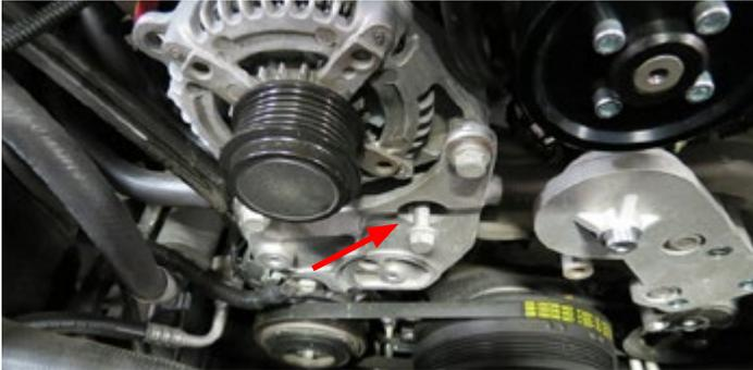
16. Apply Blue thread locker to one end of the M10 Stud from Bag #1. Thread the stud, by hand, into the alternator bracket. Using the supplied M10 nut from Bag #1, continue threading the stud into the bracket until it stops. Remove the M10 nut.
