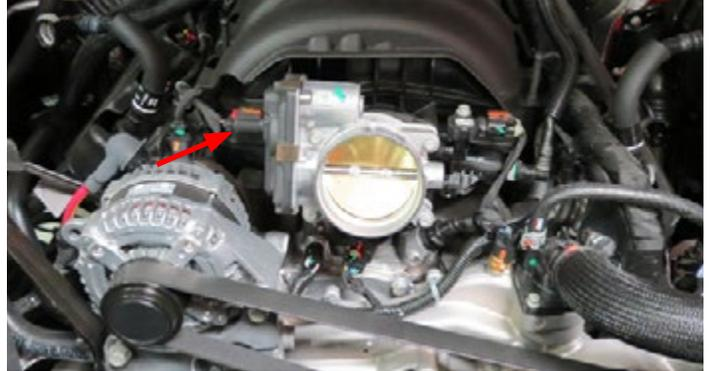
5. Unplug the MAP harness connector from the MAP sensor. Remove the EVAP hose from the EVAP solenoid and unplug the EVAP harness connector. **TIP: EVAP solenoid is located under the MAP sensor.** MAP sensor will be reused.
