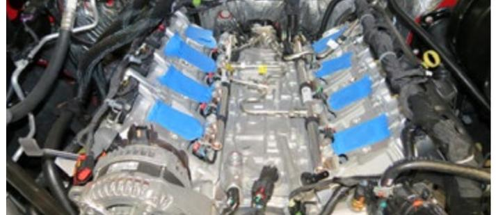
11. Using a 1/2" breaker bar, rotate the tension counterclockwise and remove the stock drive belt.
