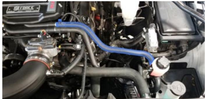
**NOTE:** The following steps demonstrate how to route the hoses to the LTR water pump. Some vehicles are equipped with a plastic shield while others will have a steel brace. If you have a steel brace, skip to step 87.
