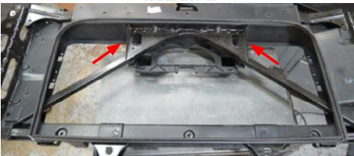
56. Using a right angle grinder, or equivalent, trim the sides of the support plate 35mm from where the plate meets the brace. The depth of the relief needs to be approximately 10mm. Deburr all sharp edges with a file and touch up relief with black paint.
