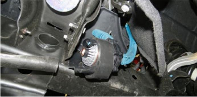
89. Using wire ties, or equivalent, secure the relay on the water pump harness to the vehicle harness mounted on the driver side firewall. Route the EVAP and water pump connectors towards the front of the vehicle following the hood latch cable. Secure the water pump harness to the factory hood latch cable loops.
