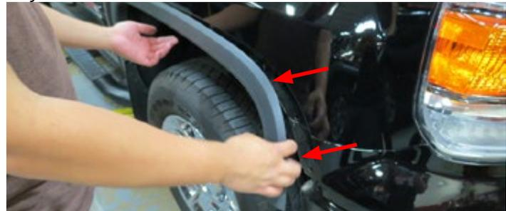
41. Using a 7mm socket, remove four (4) bolts (two per side) securing the grill assembly. **TIP: Fender lining doesn't have to be removed, but will simplify this procedure.**
