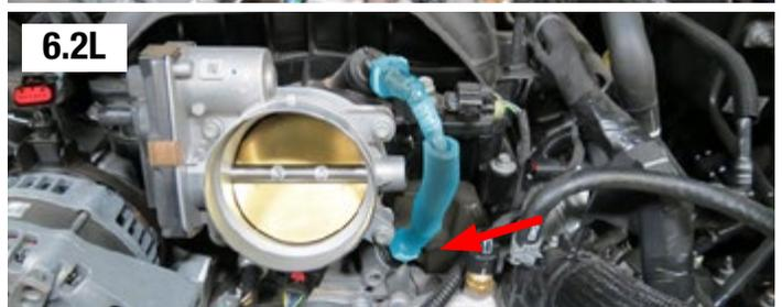
7. Detach the engine harness from the sides of the manifold cover using a panel puller. OPTIONAL: The wire ties securing the harness to the manifold cover can be removed altogether.
