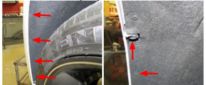
47. Using a panel puller, remove two (2) push pins (GREEN ARROW) securing the wheel well liner to the bottom of the fascia. Using a 10mm socket, remove four (4) bolts (RED ARROW) securing the wheel well liner to the bottom of the front fascia and two (2) bolts (YELLOW ARROW) securing the fascia to the chassis.
