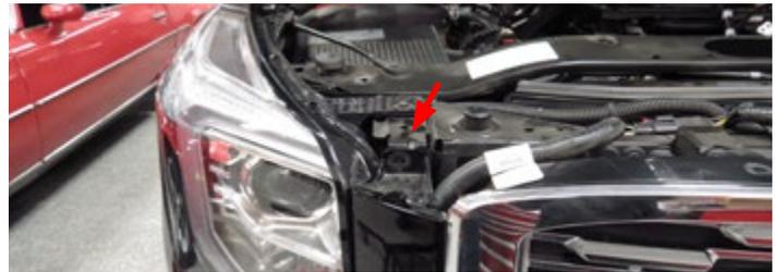
46. Using a 7mm socket remove six (6) screws, per side, securing the wheel well liner to the fascia. The wheel well liner does not have to be completely removed.
