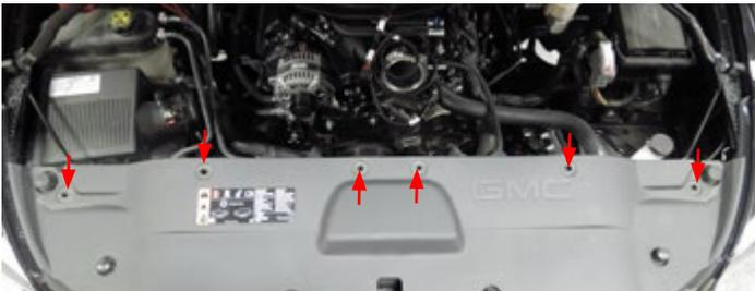
45. Using a 10mm socket, remove four (4) bolts securing the top of the grill assembly. Some applications with have two (2) more bolts located between the headlight and grille (one per side).
