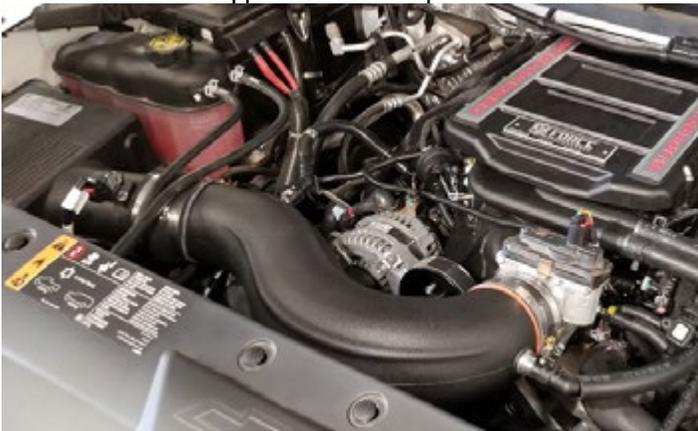
99. Install the 90° end of the supplied PCV hose to the passenger side valve cover. Install the other end to the fitting on the air inlet tube.
