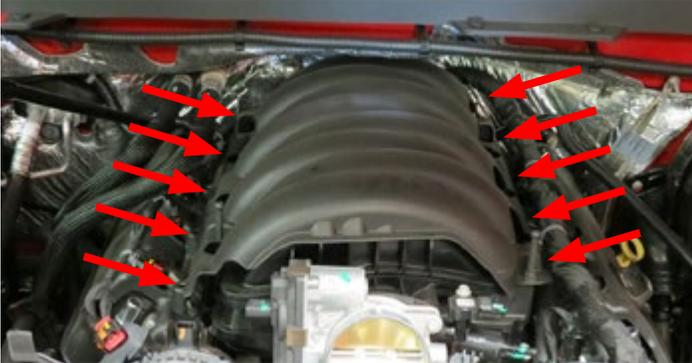
9. Using a panel puller, disengage four (4) Christmas tree push pins securing the engine harness to the rear of the manifold cover. With Christmas trees removed, carefully remove the intake manifold.
