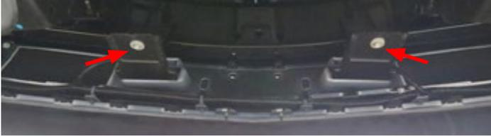
49. With the help from an assistant, carefully disengage the front fascia assembly and remove. **TIP:** Grill will detach with the fascia as an assembly.
