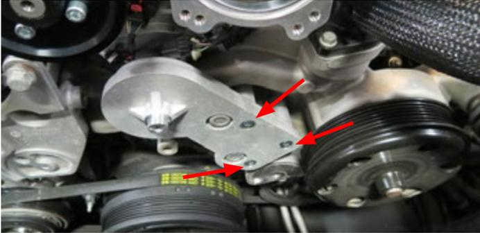
15. Remove the factory bolt securing the alternator bracket using a 15mm socket.
