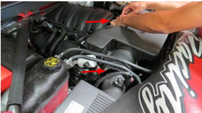
4. Unplug the throttle body harness connector from the throttle body assembly.
