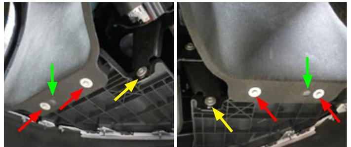
48. Using a 10mm socket, remove two (2) additional bolts securing the front fascia to the chassis.
