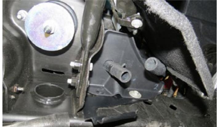
87. If the vehicle is equipped with a steel brace, route the hoses through and around the brace as shown. Use the 90° fitting and the short 90° hose provided in the kit.
