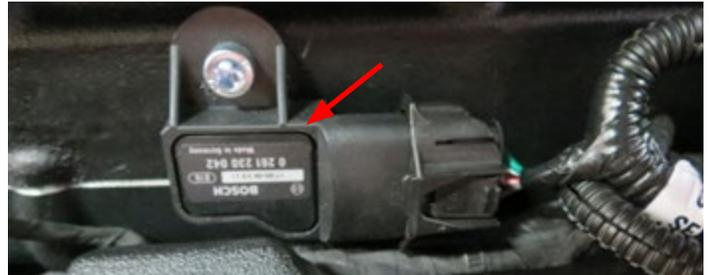
28. Remove the MAP sensor from the factory intake manifold and mount it the supercharger nose using the factory bolt. On the TMAP harness, connect the plug labeled "FACTORY MAP" to the factory MAP sensor.
