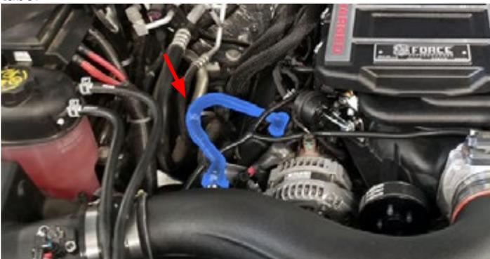
100. Install the 45° end of the supplied PCV hose to the driver side valve cover. Install the 90° end to the fitting on the air inlet tube.
