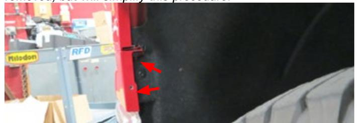
42. Remove four (4) additional bolts securing the grill assembly using a 10mm socket. **TIP:** *These need to be removed from the bottom of the vehicle.*
