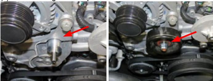
18. Insert the small pulley adapter to the backside of the supplied grooved idler pulley.
