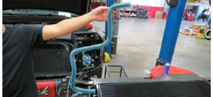
72. Install the LTR to Water Pump hose to the lower LTR barb and secure with a hose clamp from Bag #2. **TIP:** Use the hose routing diagram to reference how to clock these hoses.
