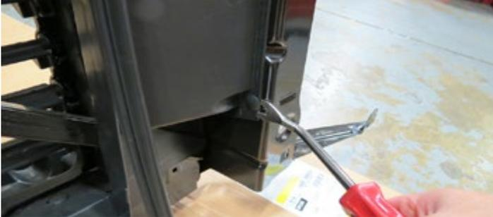
61. Position the Low Temp Radiator (LTR) on the backside of the support brace with the barbs pointing towards the driver side of the vehicle and the barbs closer towards the front of the vehicle.
