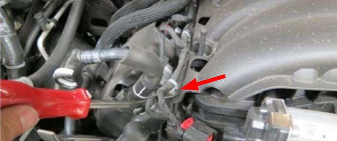
8. Using a 10mm socket, remove ten (10) bolts securing the intake manifold to the cylinder heads.
