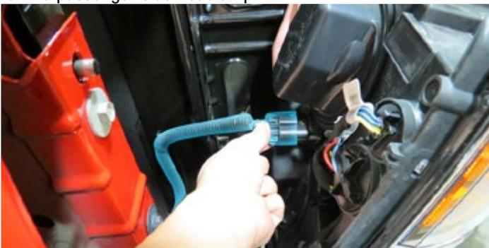
52. Unplug the ambient temperature sensor connector (GREEN). Using a 13mm socket, remove two (2) bolts securing the hood latch assembly. Remove the hood latch assembly and move aside.
