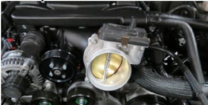
37. Connect the supplied ETC extension harness to the factory throttle body connector. Route the harness under the supercharger nose and connect to the throttle body. Secure the ETC extension harness to existing wire looms and/or hoses away from moving components and sharp edges.
