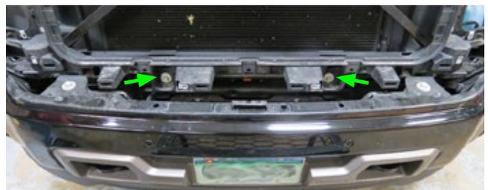
54. Use a deep 10mm socket to remove six (6) nuts (RED) and a 13mm socket to remove four (4) bolts (GREEN) securing the sides of the support brace. Carefully remove the support brace.
