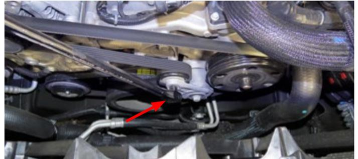
12. Using a 15mm socket, remove the factory tensioner.
