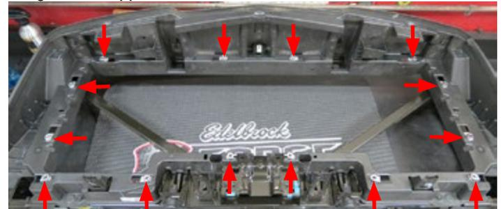
60. Using a panel puller, remove two (2) lower push pins, one on each side of the support brace.
