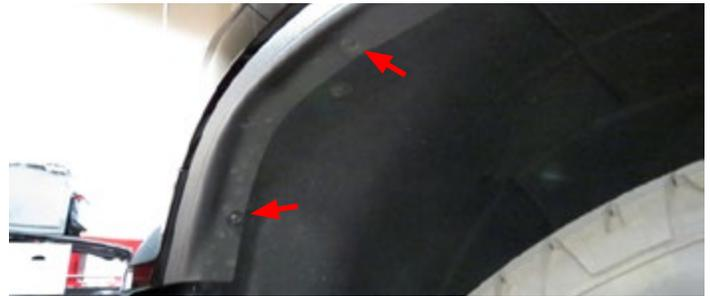
40. Carefully disengage the fender guard by dislodging the front plastic retaining clips. **TIP: Fender guard does not have to be fully removed.**
