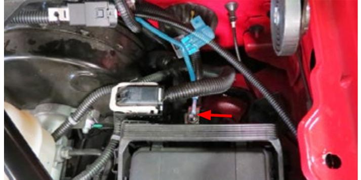
92. Route the water pump connector down towards to water pump and the EVAP connector over towards the EVAP.
