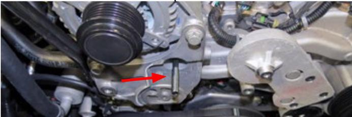
17. Place the large spacer onto the M10 Stud and secure the smooth idler pulley to the stud with one (1) M10 Washer and one (1) Nut from Bag #1. Torque nut to 18 ft-lbs.
