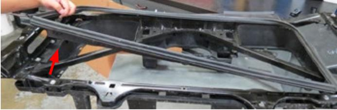
**NOTE:** There are two variants of the front support brace. Variant I has a flat support plate while Variant II has a support plate with raised sides. If you have variant II, proceed to Step 56. Otherwise disregard and proceed to Step 57.
