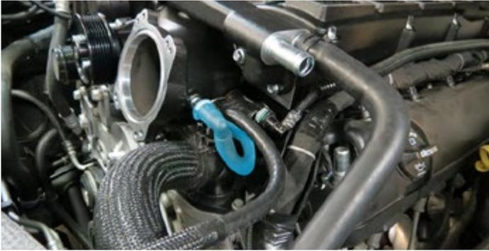
36. Using a 10mm socket, remove the throttle body from the stock manifold and install it onto the supercharger manifold using the factory bolts and the supplied throttle body O-ring gasket. **NOTE: Throttle body flange is tapped for both 5.3L and 6.2L throttle bodies. Verify proper alignment before securing the throttle body.**
