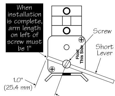
**CAUTION:** When attaching the float arm to the sender body, make sure the float ball is to the right side as you face the unit, as shown in **Diagram D**. If you attach the float arm to the left of the sender body, or backwards, the fuel gauge will read "FULL" when the tank is actually empty!
