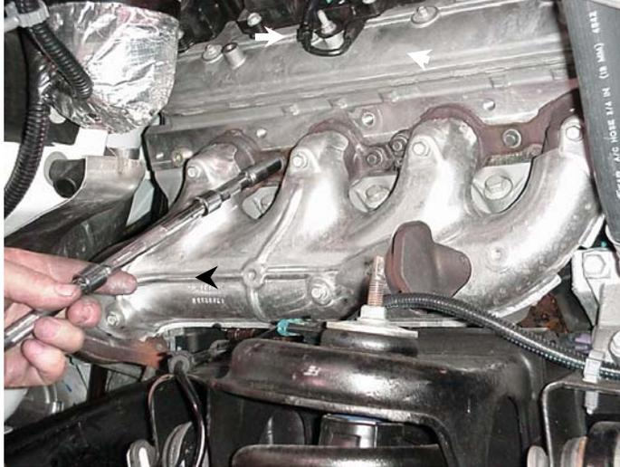
Use caution when last manifold bolt is removed as not to drop manifold
