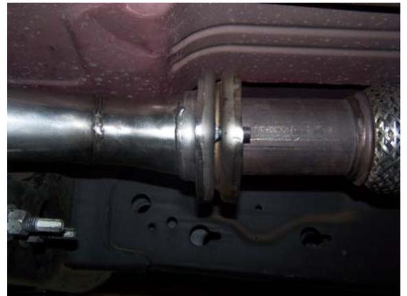
**Note: When installing the system on 2009 and up models install the provided y-pipe extension at this time. 2011 and up models with the 6.2 engine option have a 3-1/2 diameter extension pipe provided.**
