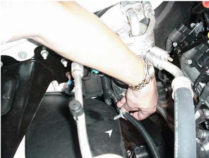
Pull barbed wire loom out of plastic inner fender panel. These need to be removed from both driver and passenger sides!
