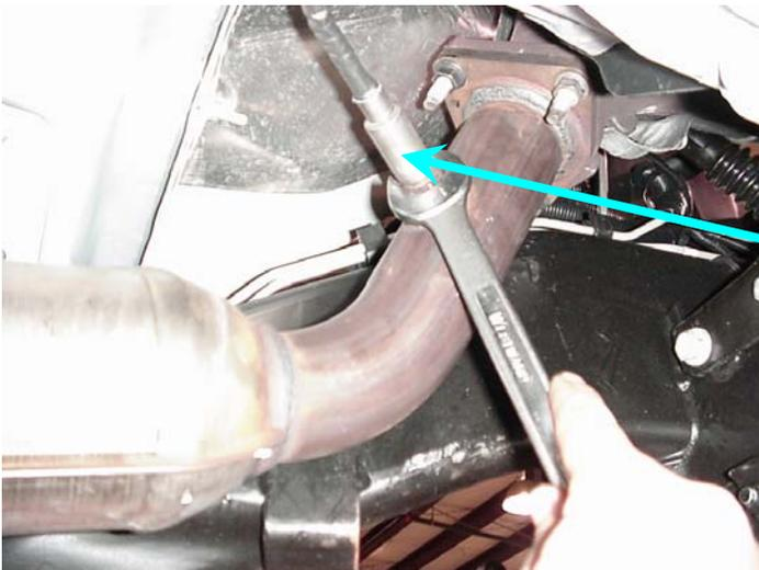
Use care in removing all four O2 sensors. Handle the sensor ends with care, keeping free from oil and dirt.
