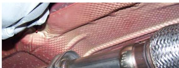
25) Driver's side catalytic converter & pipe can now be slipped into right hand pipe and attached to header collector with 3 flanged nuts. Make sure band clamp is installed over pipe before slipping left and right of "Y" together.
