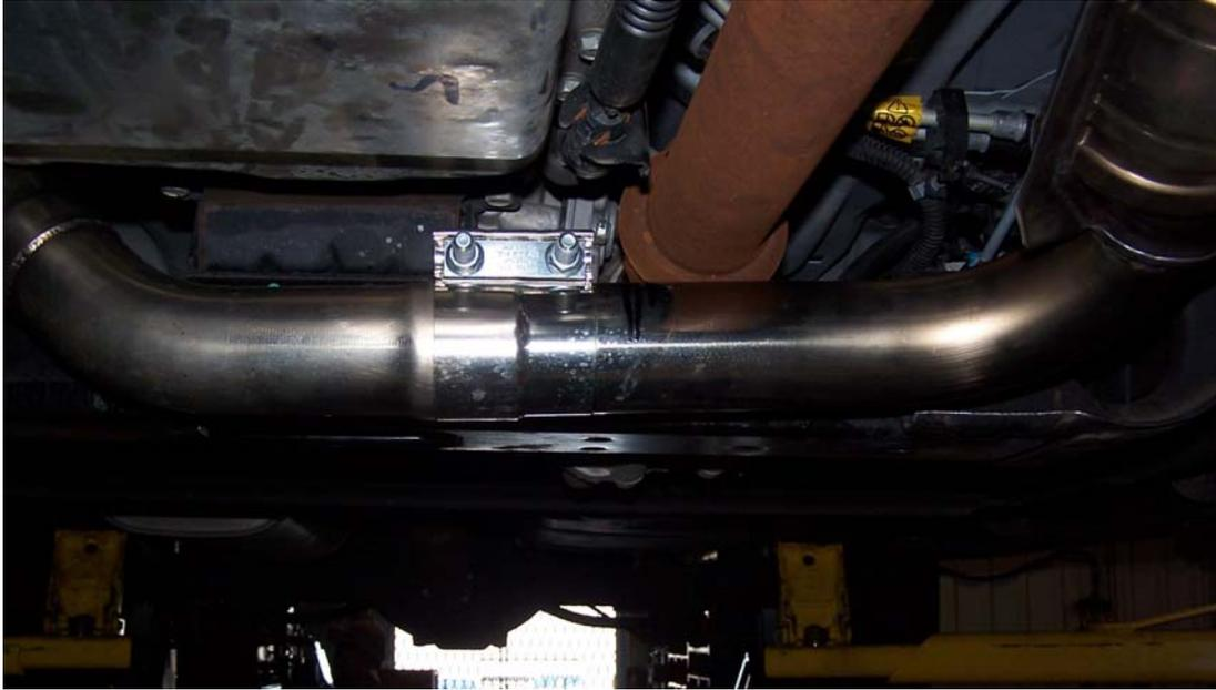
26) Raise cross member and lower transmission to install and tighten bolts.
