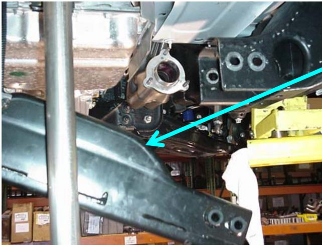
Here is the cross member lowered for removal and install.
