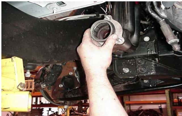
Install sintered donut gaskets before Y-pipe.
