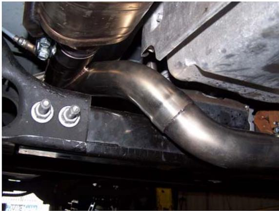
Use the single bolt band clamp to connect the catalytic converter to the "Y-Pipe".
