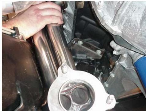
20) After installing both headers and all header bolts, brace transmission in the same manner as done in removal of stock "Y" -pipe.
