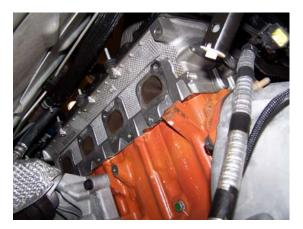
Remove the three nuts (two at the rear and one in the front) of the starter heat shield and remove the shield.
