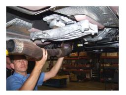
Spray the down tube nuts on the right (passenger) side with penetrating fluid and let soak. Remove the nuts.
