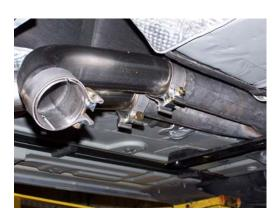
Slip the "B" section of the right (passenger) side interim tube into the passenger side inlet tube of the stock muffler. It may be necessary to enlarge the tube slightly because it has already been clamped. This can be easily done with a hand tailpipe expander available for sale or rent at AutoZone stores or similar parts outlets.
