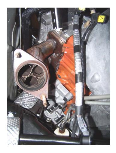
Loosen and remove all of the manifold bolts on the left side and lower the manifold and gasket out the bottom of the engine bay. This is easier said than done. The lower rear three bolts are fairly straightforward. Loosen and remove the center two bolts on the left (driver side) engine bank. Loosen and remove the top rear bolt. The top forward bolts present more of a problem. Follow the steps below to get to them.
