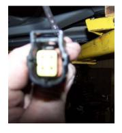
Note: O2 sensors are delicate electronic components and should be handled very carefully. Take extra care in not contaminating the sensing end with shop towel lint, finger prints, oil, etc.
