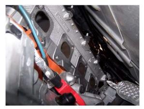
Begin the left (driver) side header installation by finding and preparing eight of the supplied header bolts by putting a small amount of anti-seize on each of the eight (8) bolts required for the left side. Slip a bolt through the lower holes in the OEM style stainless steel gasket as shown below. Make sure that you hand start each bolt to prevent cross threading during installation.
