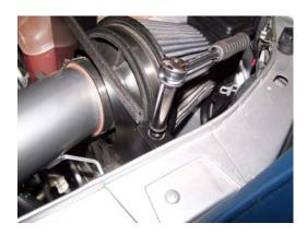
Loosen and remove the bolt securing the cold air box baffle.
