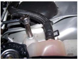
Deflect the small plastic tab on the coolant reservoir and pull the power steering oil tank upward to disengage it from the coolant tank. Then remove the two bolts holding the coolant tank to the inner fender and push the tank toward the windshield. From this point you can reach the remainder of the upper manifold bolts by slipping your hand and wrench between the head and the inner fender.  When all bolts are removed the manifold can be removed from the bottom of the vehicle.
