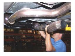
Note: O2 sensors are delicate electronic components and should be handled very carefully. Take extra care in not contaminating the sensing end with shop towel lint, finger prints, oil, etc.
