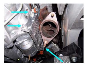
Loosen and remove all of the manifold bolts on the right side. As with the
