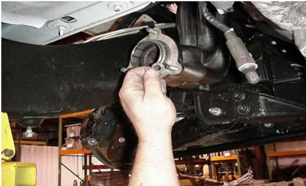
Install one spacer per stud. This prevents the gasket from being crushed beyond its intended yield point as the catalytic converters and “Y”-pipe are being tightened into position. ( Do this on both headers )
