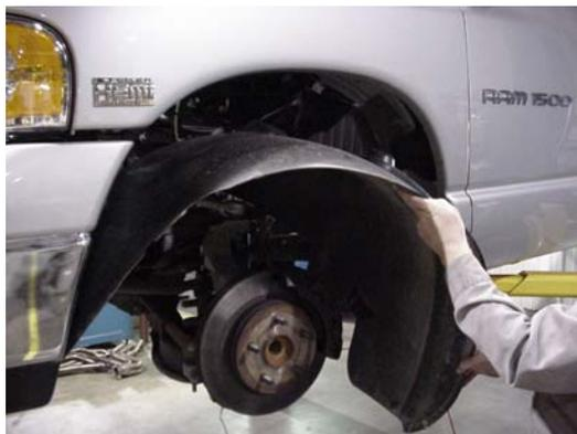
Install panels and screws in the same manner in which they were removed.
