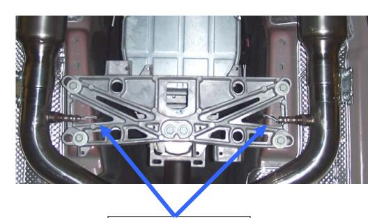
Rear sensors cable routing
