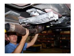
Spray the down tube nuts on the right (passenger) side with penetrating fluid and let soak. Remove the nuts. Note in the picture that the right side has a heat shield that is held on by the first of two sets of nuts.
