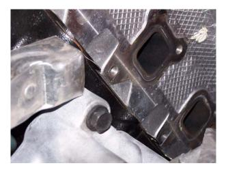
• Begin the left (driver) side header installation by finding and preparing enough of the supplied header bolts by putting a small amount of anti-seize on each of the eight (8) bolts required for the left side. Slip a bolt through the lower holes in the OEM style stainless steel gasket as shown below. Make sure that you hand start each bolt to prevent cross threading during installation.
