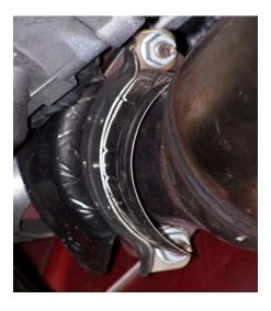
Pull the stock catalytic converter down and off the cast manifold studs
