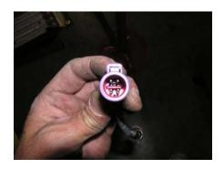
Notice the connectors with the external tabs removed to allow for plug in.
