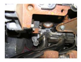
Locate two of the O2 sensor extension cables. Use these extensions to plug into the front and rear O2 sensor connectors on the left (driver) side in the vehicle wiring harness.
