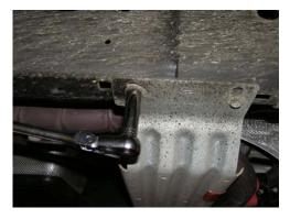
Next, loosen the nuts on the clamp between the stock "Y"-pipe and the
