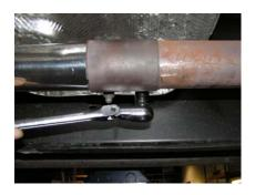
Note: O2 sensors are delicate electronic components and should be handled very carefully. Take extra care in not contaminating the sensing end with shop towel lint, finger prints, oil, etc.
