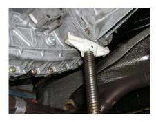
Now that the transmission is properly supported, loosen and remove the four (4) bolts that hold the cross-member to the frame.
