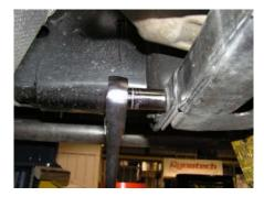
Now that the cross-member has been removed, loosen but do not remove the nuts (2 on each side) on both the left and right side down tubes where the exhaust system is attached to the stock cast manifolds. The picture below shows the driveshaft of the 4WD model which may or may not be in your vehicle.
