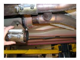
The "X"-pipe assembly should be completely free to remove at this point.
