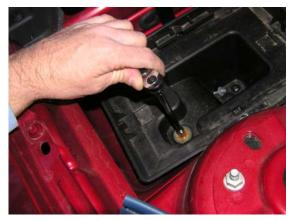
Page 5 of 17 Lit1005 Rev 1 Rev 3  Slide the red retainer clip out on the MAF (Mass Air Flow) sensor and disconnect the harness.
