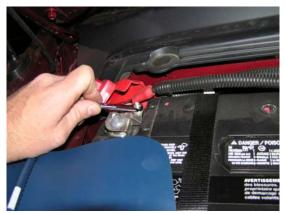
Removal of the battery and tray provides more room to get to the manifold bolts during a later step. Remove the battery cover and tie-down, the battery, and finally remove the battery tray by removing the 3 bolts holding the tray in position.
