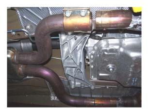
Remove the manifolds at this time. Once removed, remove the front 02 sensors. Be careful not to ruin the threads during removal. Threads have been known to gall during removal. If this occurs, your only choice is to replace it or them with new ones. As each sensor is removed, mark it accordingly so that it may be replaced in the same location during reassembly.
