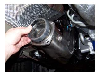
Lower the front of exhaust down to allow room to install powers cats.
