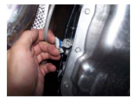
Page 6 of 11 Lit 1018 v2 After removing the rear O2 sensors, loosen the nuts on the clamps that
