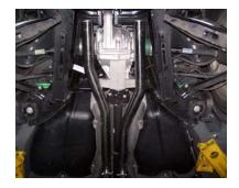
Install muffler inlet tubes into rear interim tubes and tighten band clamps so they are self supported but not fully tightened. Also install rear gaskets between muffler inlet tubes and mufflers. Bolt muffler inlet tubes onto mufflers and install rear rubber hangers onto muffler inlet tubes.
