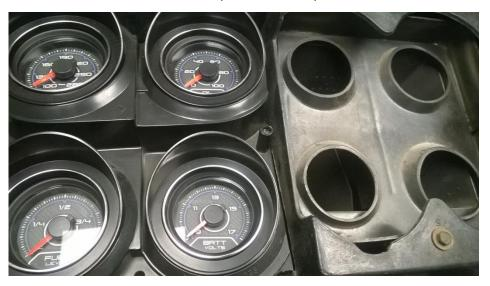
Install the panels to the dash using the screws provided
