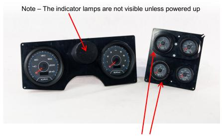
When installing gauges into the panel, place spacers provided onto (2) left side 2 1/16" gauges between gauge bezel and panel
