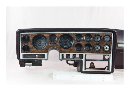
Remove the 7 screws that hold on the front bezel assembly. (under the dash brow). Remove the front bezel. Retain screws for use in re-installation of bezel.
