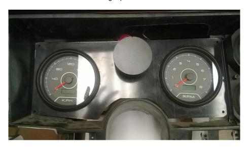
Install the black spacer/block out plate
