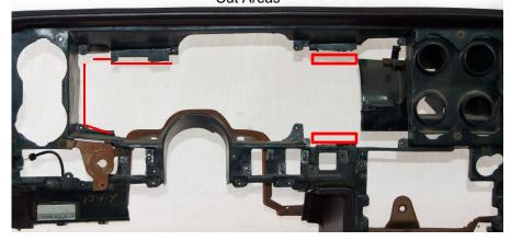
Dash is ready for panel installation. Install panel with (4) 2 1/16 first.
