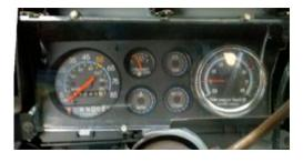
Remove lens/plate and original gauges (not re-used)
