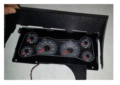
Assemble blockout and install on gauge assembly. The notches lock in and should be sturdy once inserted. Adhesive is optional.
