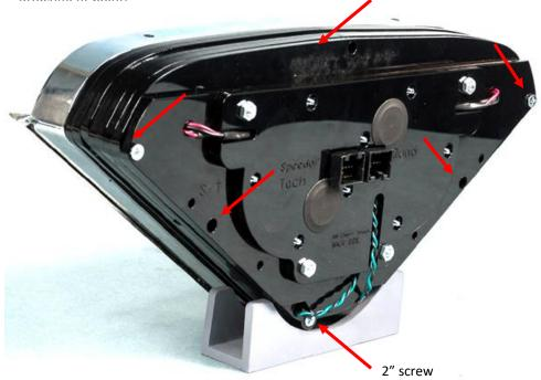
Wire according to the following diagram (next page) plug corresponding plugs into the ports on the back. They are labelled by engraving. The plug on the "QUAD" side has access to change the DIP switches for your fuel range. The stock range is 0-30 ohm.
