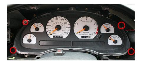
Carefully pull the cluster slightly forward and tilt it back and upwards allowing room to remove the wiring harness/plugs
