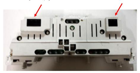
Disconnect the two harness connecters from the backside of the cluster.
