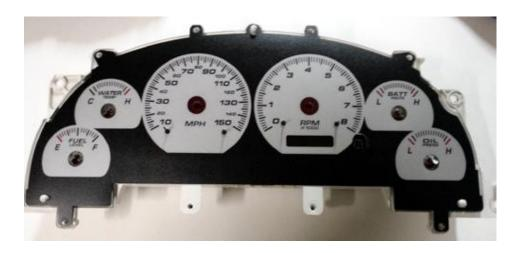
Install pointer stops by snapping into holes cut into overlay
