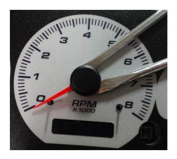
Pull original overlay off of cluster, it is heat staked to the clear refractor in several places. Just rip it off. Any remnants of the original overlay will need to be removed so that the surface is flat.
