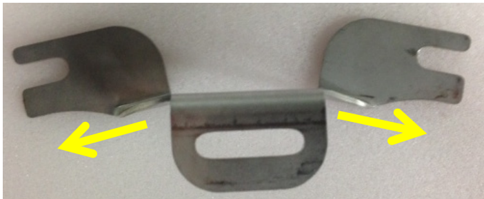
MTBRGMK – After Bending (Bend at thin sections)
