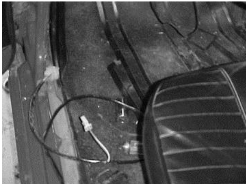
Figure 8.6 Driver Kick Panel and Jamb Routing
