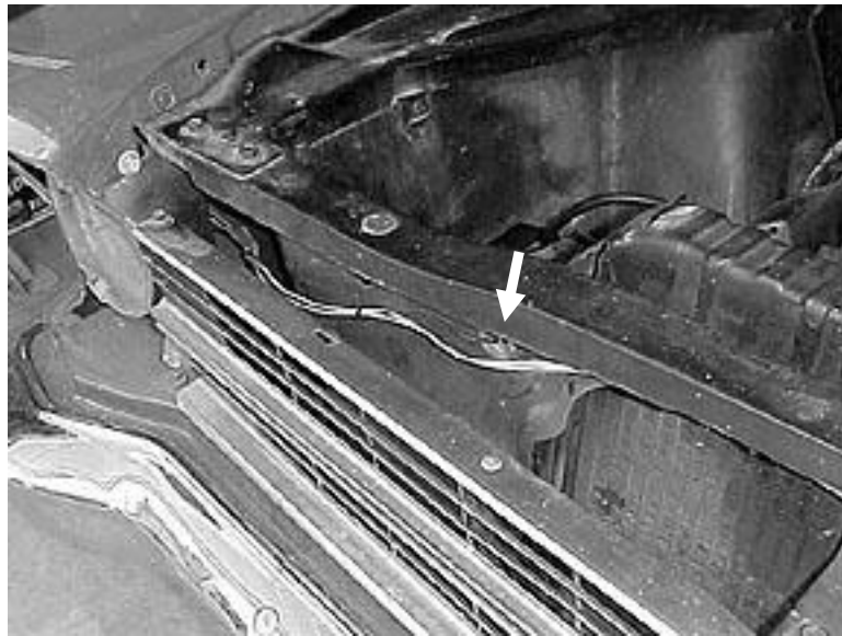
Figure 8.19 Passenger Side Headlight Wire Routing
