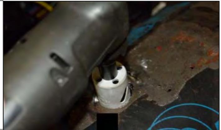
17. From underneath the vehicle, install the B&M selector lever in position on the transmission. Re-use the stock selector lever nut. Torque the nut to 23ft.lbs. The lever should move smoothly from front to back with a positive click in each gear position.
