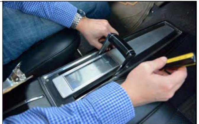
3. Lift the shift indicator assembly from the console, unplug the two (2) bulb harnesses from the shift indicator assembly and set aside.
