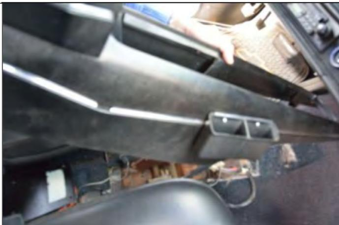
11. Remove shifter cable retaining clip.
