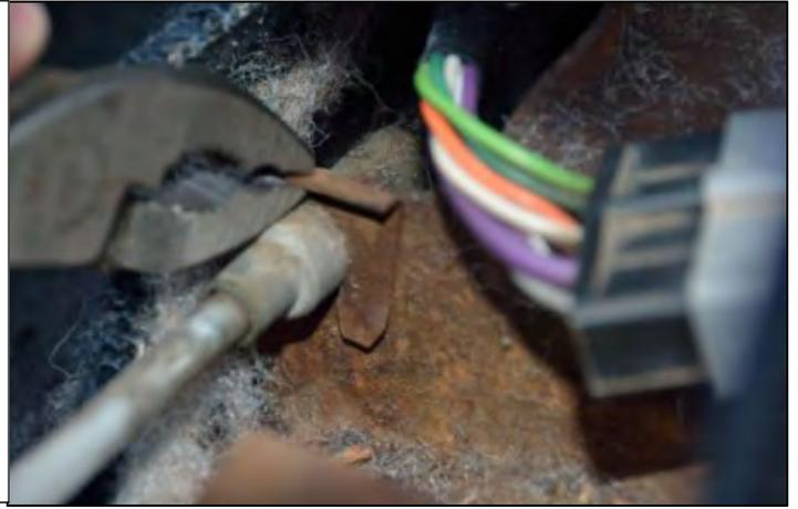
12. Remove the retaining clip that is securing the end of the shifter cable to the shifter. Then remove the cable from the shifter.
