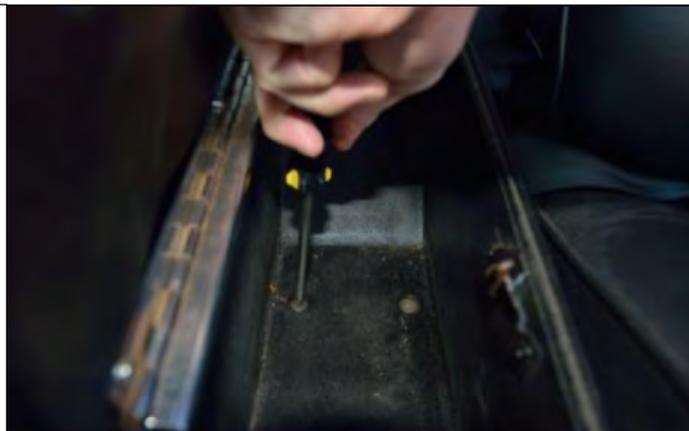
8. Disconnect the electrical harnesses from the shifter module: Neutral Safety Switch, Reverse Back-Up Light connectors.
