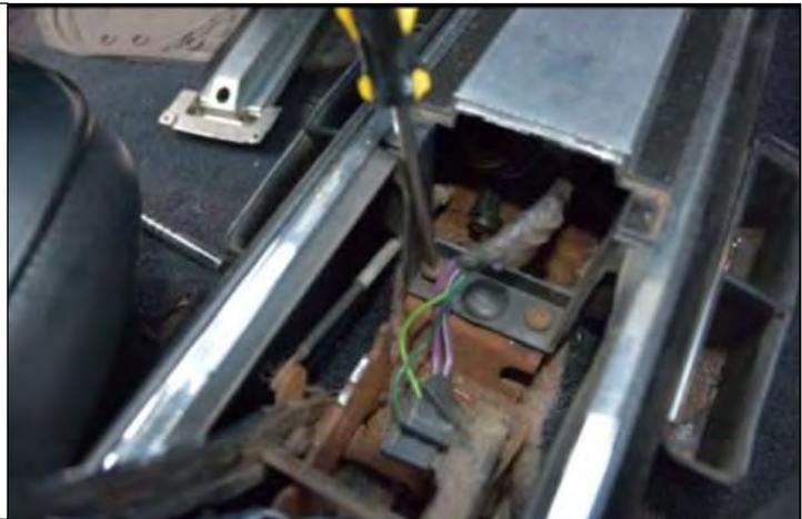
6. Remove the two (2) screws that are securing the front end of the console to the floor.
