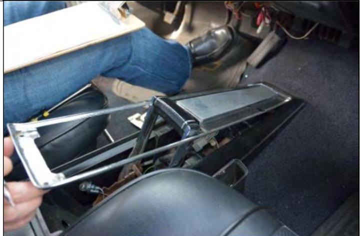
5. Remove the two (2) screws that are securing the center of the console to the shifter.
