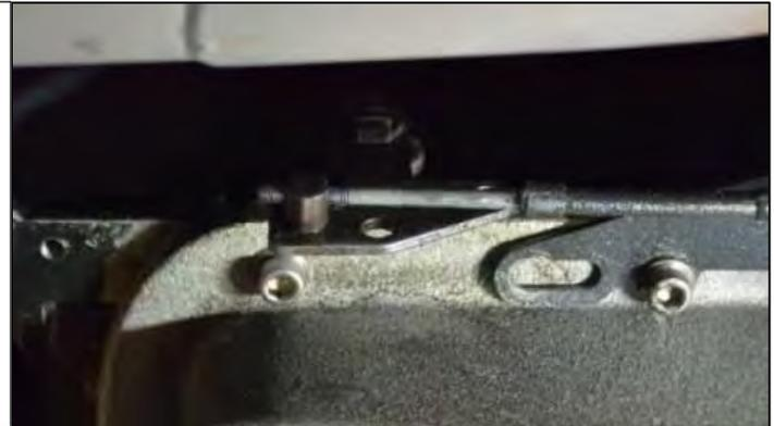
18. Remove the two transmission oil pan bolts from the middle of the left side of the oil pan. Install the cable bracket in position. The bracket must be installed with spacers between the pan and the bracket. Install two 5/16 x 1.00" bolts (or M8 x 25 mm for metric transmissions) supplied and tighten 12-13 ft. lbs. Do not overtighten as this can damage the pan gasket.
