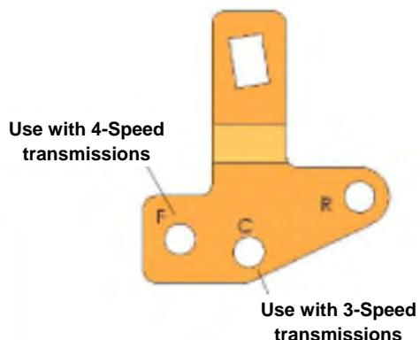
Leave the swivel out of the hole and move the selector lever to Park, all the way forward. Also move the shifter to Park position. (See operation section, page 8). Reinsert the swivel into the hole in the selector lever. Check to see that the swivel will slide freely in and out of the hole in the selector lever in this position. If it does not slip in freely, adjust the swivel slightly until it will slip into the hole in the lever.
