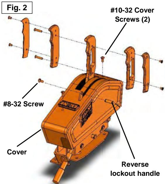
38. Re-install the side plates and side-grips onto the stick securely with the six #6-32 screws. Secure the carpet to the floorboard and the door edges. Your shifter is now ready to use.
