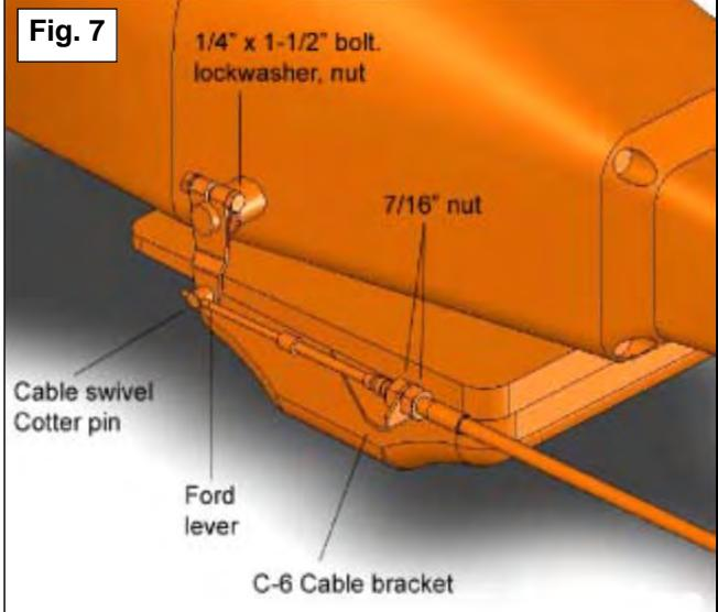
20. Remove the two transmission oil pan bolts directly below the shift lever. Install the cable bracket into position with two spacers between the pan and the bracket (See Figure 7). (If your transmission is equipped with a cast aluminum oil pan these spacers can be omitted). Install the two supplied 5/16-18 x 1.00" pan bolts and tighten to 12-13ft.lbs. Do not overtighten as this can damage the pan gasket.
