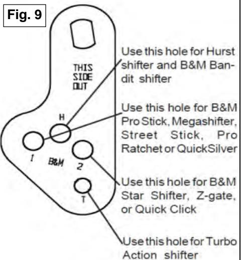
Leave the swivel out of the hole and move the selector lever to Park, all the way forward. Also ratchet the shifter to Park position (all the way forward). Reinsert the swivel into the B&M1 hole in the selector lever. Check to see that the swivel will slide freely in and out of the B&M1 hole in the selector lever in this position. If it does not slip in freely, adjust the swivel slightly until it will slip into the **B&M1** hole in the lever.
