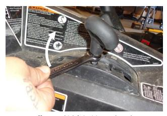
1. <u>Turn off your vehicle's ignition and set the</u> <u>parking brake</u>. Loosen the jam nut under the stock shifter handle.
