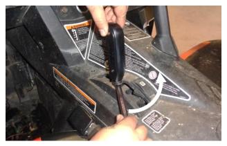
4. Hold the Magnum Grip Shifter Handle in the desired position and tighten the jam nut.
