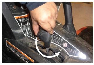
2. Unscrew the stock shifter handle from the shifter lever.
