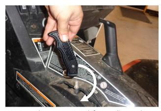
3. Screw the Magnum Grip Shifter Handle onto the shifter lever. (Avoid cross-threading.)
