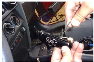
4. On the transfer case shifter handle assembly (1), back out the four screws until their heads extend slightly above the handle surface.
