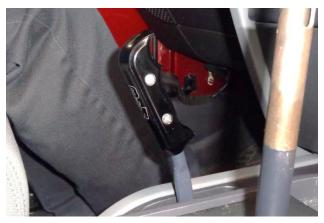
Install the handle on the transfer case shift lever. Align the handle as desired, then tighten the four screws.
