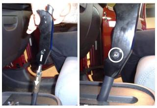
6. On the main shifter handle assembly (2), remove the left handle cover. Install the handle on the shift lever, and align the handle and lever screw holes.
