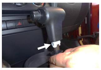
Remove the screw at the base of the shifter handle and remove the handle from the lever.
