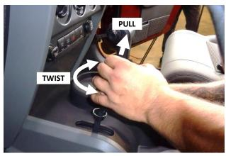
2. Grab the transfer case shifter handle firmly with both hands. Twist the handle side to side while pulling straight up to remove it from its lever.
