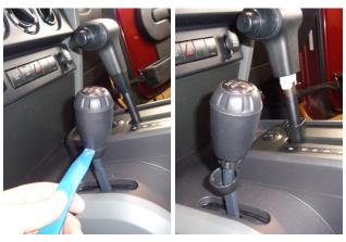
1. Use a plastic trim tool to separate the trim ring from the bottom of each shifter handle.
