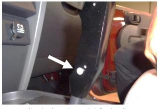
7. Install and tighten the stock shifter handle screw (removed at Step 3).
