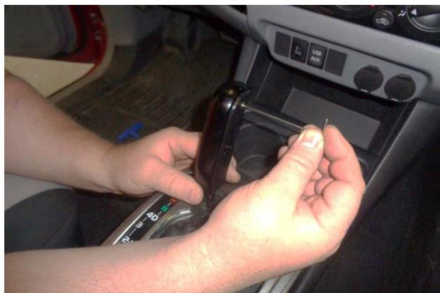
5. Install the left and right side plates (2) and (3) with the 4 flathead screws (4). (Two screws each side.)
