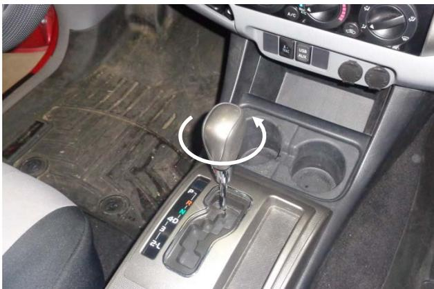
1. **Turn off your vehicle's ignition and set the parking brake.** Remove the stock shifter handle by rotating it counter-clockwise on the shifter stick.
