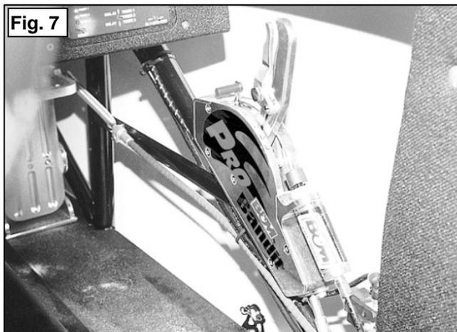
9. At this stage the shifter cable, the neutral safety switch and the air slave cylinder should be installed. Before you proceed with mocking up the B&M *Pro Bandit Shifter* in your vehicle, temporarily reinstall the side cover with the center screw only. This is to insure that the gate plate and the mechanism do not move from the inside of the shifter body when you are positioning it in your vehicle. You are now ready to locate your B&M *Pro Bandit Shifter* in your vehicle.
