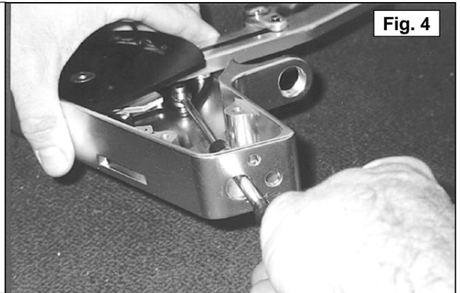
5. Push the cable anchor tab flush to the rear of the shifter body. Align the 17/64" cable flange hole with the 9/32" hole in the shifter body. Be sure to use the hole directly above the large cable access hole. Install the 1/4" bolt from the outside of the shifter body through the cable mounting flange until the bolt sticks through to the inside of the shifter body. Place the supplied 1/4" washer over the exposed threads on the inside, then thread on the 1/4" nut and tighten (See Figure 5).
