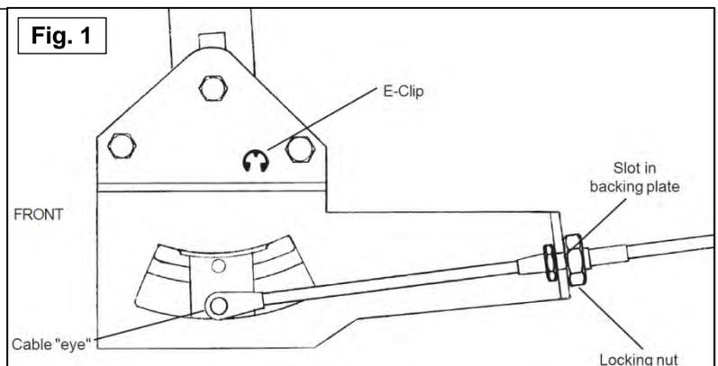
7. Check that the shifter moves through all the gear positions and that the other end of the cable moves in and out. Route the cable to the transmission as shown in Figure 2 to avoid sharp bends or damage to the cable. For GM and Ford transmissions route the cable to the transmission from the rear. For Chrysler transmissions the cable must be looped around to the front side of the transmission.
