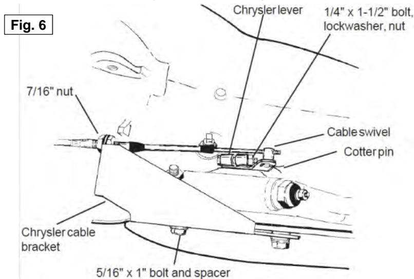
20. Remove the two transmission oil pan bolts directly below the shift lever. Install the cable bracket in position (See Figure 6) with two spacers between the pan and the bracket. (If your transmission is equipped with a cast aluminum oil pan these spacers can be omitted.) Install the two 5/16-18 x 1.00" pan bolts supplied and tighten to 12-13ft.lbs. Do not overtighten as this can damage the pan gasket.
