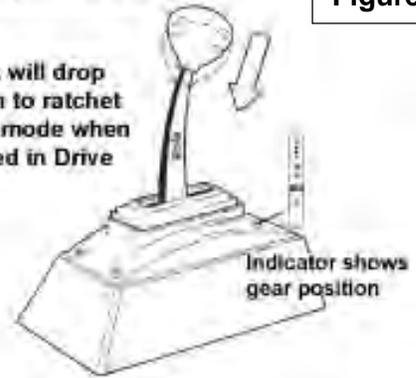
**Shifting in the ratchet mode:** Move the stick forwards or backwards with a quick firm action until it hits the internal stop.
