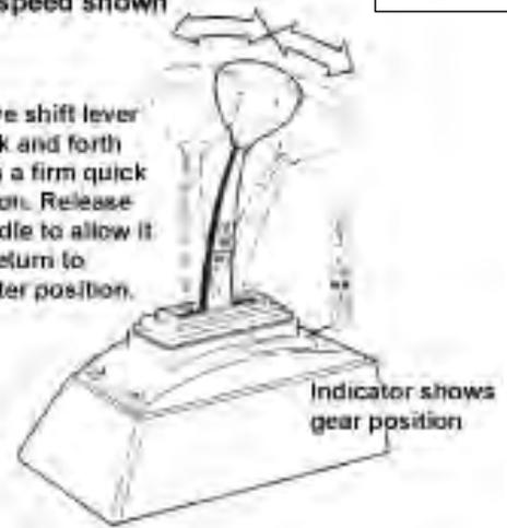
To switch the shifter from ratchet mode back to straight gate operation, ratchet the shifter to the Drive position and pull up firmly on the knob. You are now in the straight gate mode, still in Drive (See Figure 11). Remember: To go from straight gate mode into ratchet shift mode or from ratchet mode into straight gate mode the shifter must be put into the Drive position.
