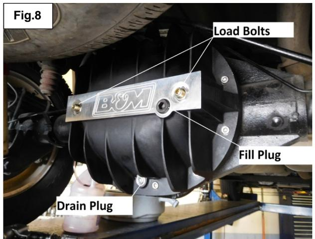
20. Install the supplied 1/2" NPT fill plug on the B&M Cast Aluminum Rear End Cover and tighten.
