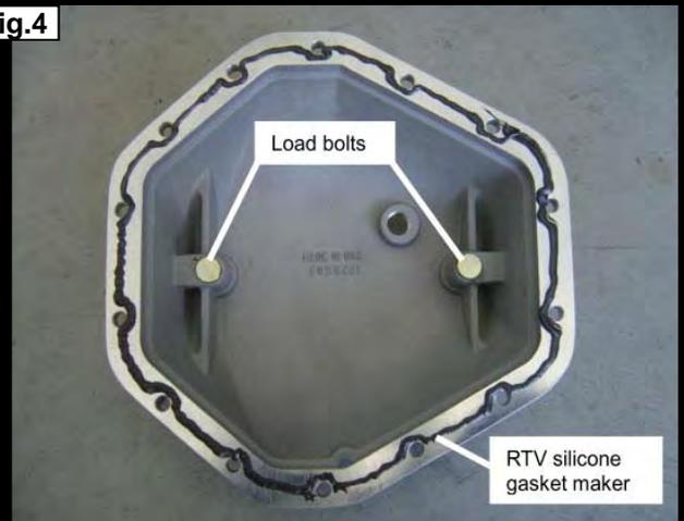
12. Apply a bead of RTV silicone gasket maker to the B&M Cast Aluminum Rear End Cover. Run the bead inside the bolt holes (See Figure 4).
