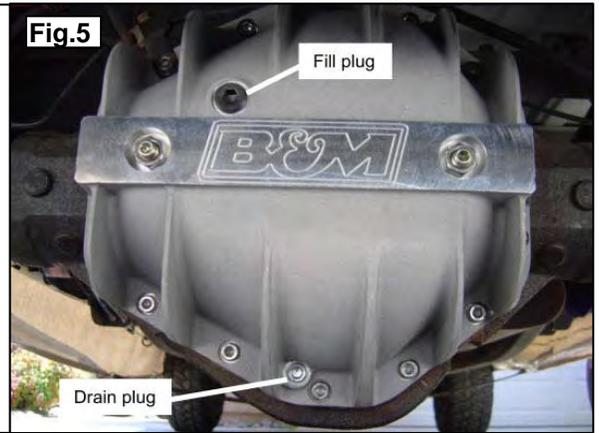
20. Install the axle housing fill plug and torque to 20ft.lb.
