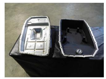
3. Install the 1/8 accessory pipe plug and then install the drain plug, be sure to use thread tape on the drain plug threads.
