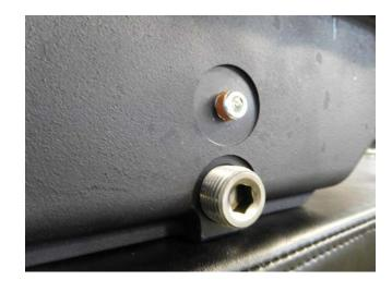
4. Inspect and wipe clean the stock oil pan gasket. If the gasket is in good condition, it can be re-used.
