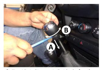
2. Use a trim tool to separate the trim ring from the bottom of the gearshift knob (A). Remove the knob by grasping it firmly with both hands and rotating it back and forth slightly (B) while sharply pulling it straight up. Finally, remove the trim ring from the shift lever. Repeat to remove the shift knob and trim ring from the transfer case.
