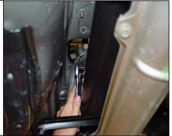
11. Remove shifter from car. (Metal plate and spring will be used on new shifter)
