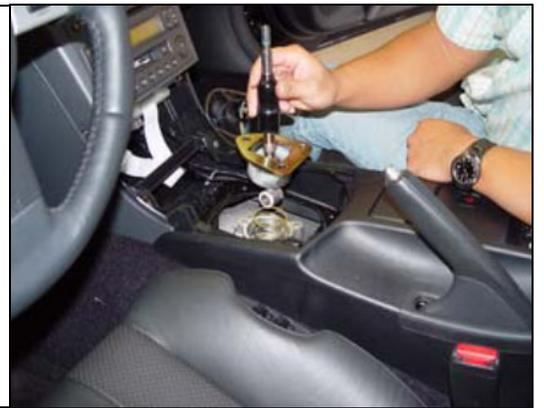
12. File out approx. .125" from shifter casting in indicated area. Clean out metal chips and relube entire pocket with provided grease.
