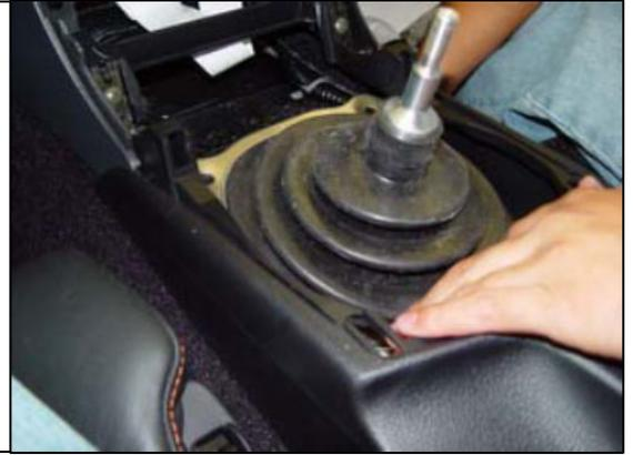
23. Reinstall white foam (350Z and G35 only) and console plate, making sure to re-plug in wiring harness.
