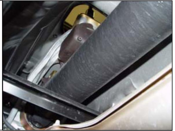
19. Adjust shifter plate so that reverse pin rides on the stock plate while going into 6th gear. Shifter should need to be pushed down to engage reverse. Evenly torque bolts to 10lbs-ft (13.6Nm). Test movement of shifter into all gears. DO NOT operate vehicle until all gears can be fully engaged smoothly.
