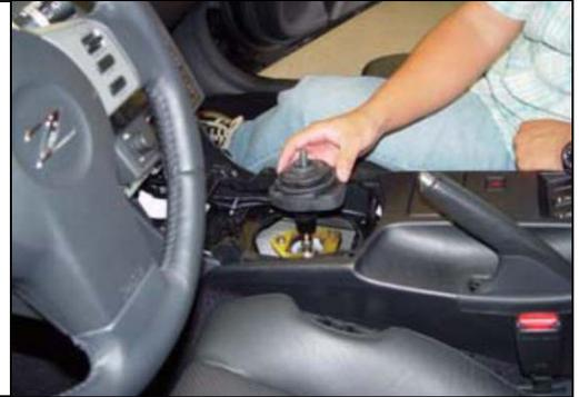
7. Remove bolts holding down metal shifter plate.
