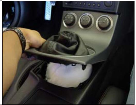
3. Unplug wiring harness from console plate and remove console plate.
