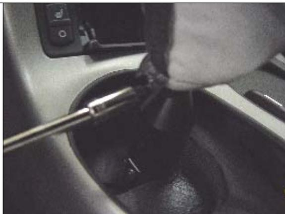
**STEP 19.** Remove foam and (4) nuts securing rubber.
