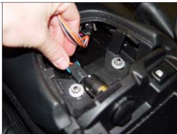
**STEP 6.** Remove panel next to ignition key (temperature sensor) and remove screw.
