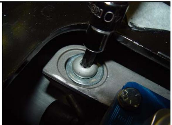
**STEP F.** Remove "L" pin from pin hole and test shifter through each gear.
