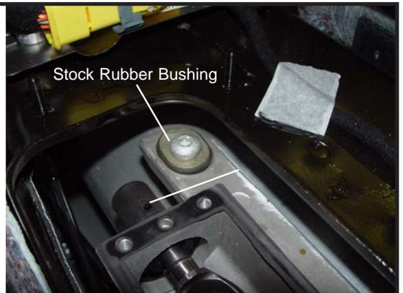
**STEP A.** See top-right picture for indication of working area. Remove "L" pin from the stock shifter. With the shifter still in neutral and E-brake in the ON position, insert the "L" pin into the pin hole of the shifter base. The "L" pin is used to keep everything aligned. If done correctly, shifter should not be able to shift out of neutral position.
