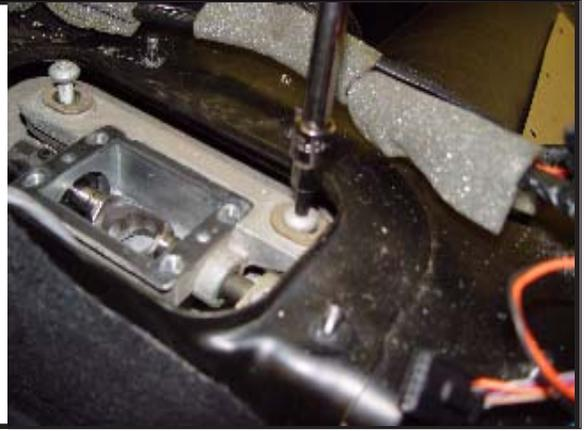
**STEP C.** Remove stock rubber bushings and spacer.
