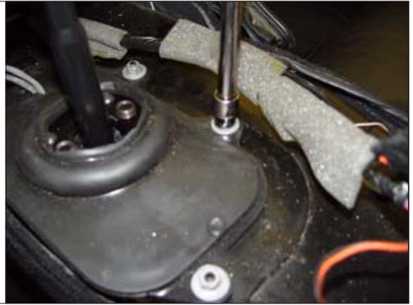
**STEP 20.** Remove (4) bolts securing shifter and remove from vehicle.
