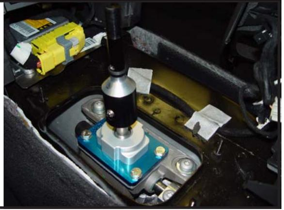
**STEP 25.** Reinstall foam and (4) nuts securing rubber.
