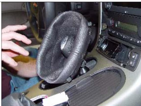
**STEP 18.** Remove screw securing knob and lift out front center console. Be sure to remove connector wires.
