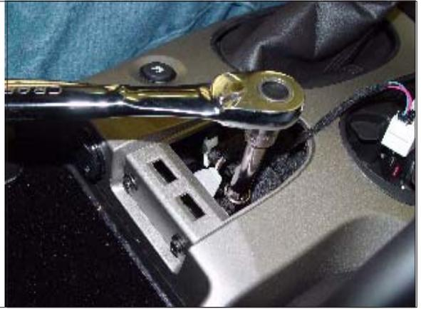
**STEP 12.** Remove (4) bolts securing arm rest and remove arm rest.
