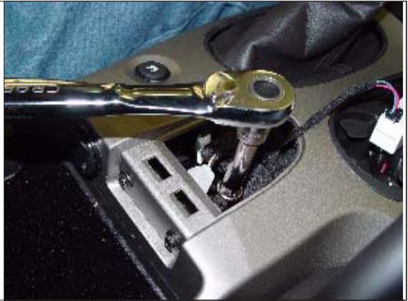
**STEP 32.** Reinstall (2) screws under passenger airbag panel.
