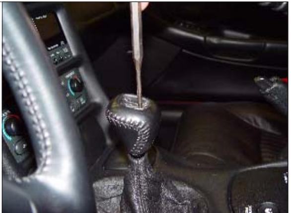
**STEP 43.** Ensure that all gears can be smoothly and fully engaged without binding or rough movement. Correct any problems prior to operating the vehicle.
