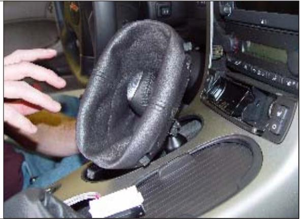
**STEP 28.** Reinstall passenger side panel and lift up on front center console.
