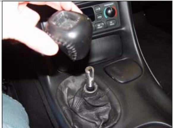
**STEP 42.** Reinstall metal insert into knob and shift pattern indicator.
