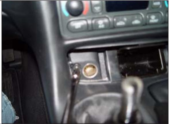
**STEP 8.** Remove small inserts at rear of rear center console and remove (2) nuts.
