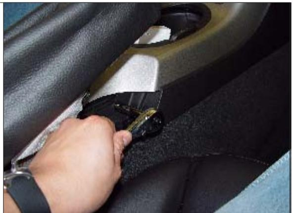
**STEP 30.** Reinstall sleeve around emergency brake.
