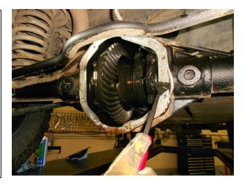
8. Screw in the load bolts from the inside of the cover until they make contact with the boss, then next apply a bead of RTV silicone gasket maker to the B&M differential cover. Run the bead inside the bolt holes. If your vehicle has a reusable gasket it may be reused but check condition of it.
