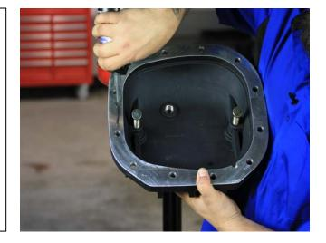
9. Install the B&M differential cover on the axle housing using the 3 OE/stock studs on top right side of cover & the supplied allen bolts and washers. The original stud fasteners are required to accommodate the factory wiring clips/brackets clips/brackets. Torque to factory specs.
