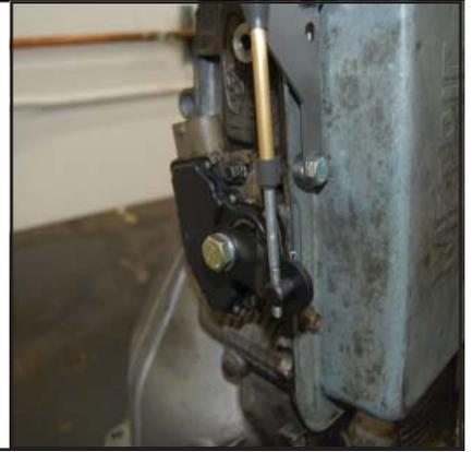
STEP 21. Start the engine and shift the transmission through all of the gear positions and then to neutral. Check the transmission fluid level, and add more fluid if necessary to bring it up to the proper level. Be sure that the shifter operates smoothly and that the transmission shifts to the correct gear.
