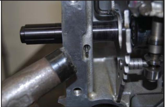
STEP 11. Install Detent Spring.
