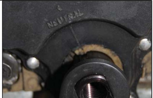
STEP 15. Secure B&M Selector Lever onto B&M Selector Shaft with M10 bolt and M10 washer.
