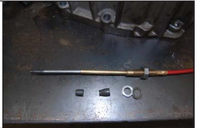
STEP 18. Route the cable from the shifter to the transmission as explained in the shifter installation instructions. Avoid sharp bends and route the cable away from the hot engine exhaust parts. Cable may be secured up and out of the way with nylon cable ties.
