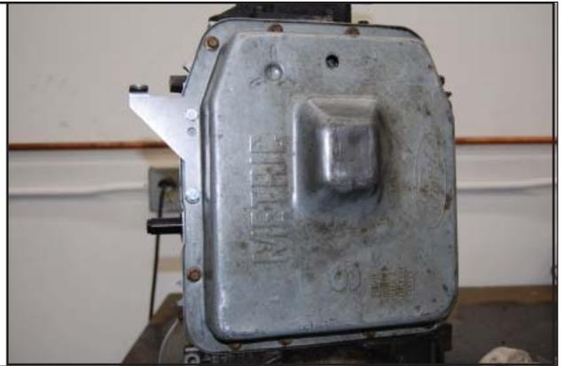
STEP 14. With selector shaft in neutral position, Install Neutral Position Sensor. (NOTE: replace Neutral Position Sensor in same orientation as found before removal). Align sensor to neutral position before tightening two (2) 8mm bolts.
