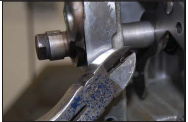
STEP 7. Remove nut on inner end of shaft.
