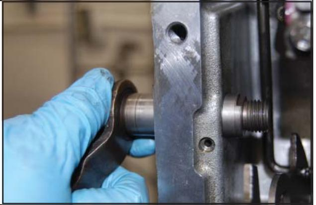
STEP 9. Slide B&M Selector Shaft into case. Engage B&M Shaft with inner shift lever and install nut. Use B&M Selector Lever to visualize position of selector shaft.
