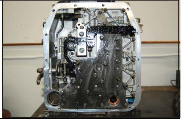
STEP 5. Remove one (1) bolt and remove detent spring.
