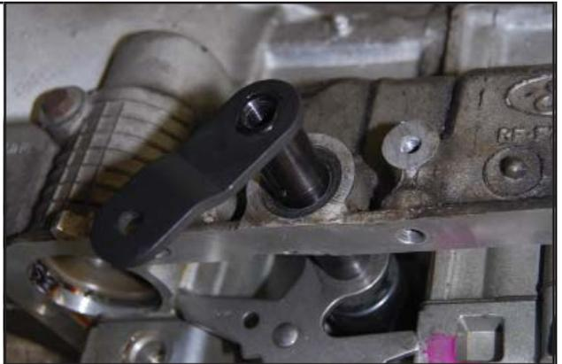
STEP 10. Install Selector Lever Retaining Pin.
