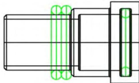
5. Lubricate the O-rings with ATF and push the extension tube onto the transmission end of your stock oil pick-up tube. Push the extension tube onto the pick-up tube until it stops against the shoulder on the pick-up tube.
