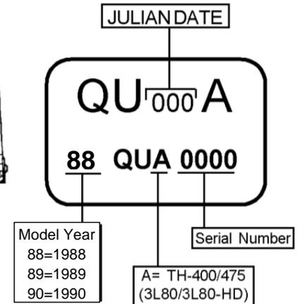
If the I.D. tag is unreadable or missing you will have to remove the oil pan and valve body from the transmission to determine if your transmission has an early or late style case (See Fig. 2). The manufacturing date check applies only to 1988 transmissions, this kit will work correctly in all subsequent application years specified in the heading of these instructions.
