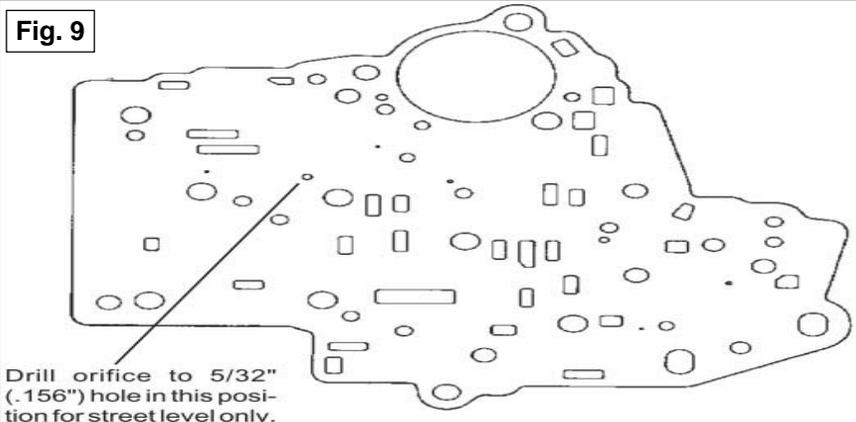
8. Thoroughly clean the valve body and separator plate in clean solvent to remove any contamination. Remove any old gasket material stuck on the valve body channel surface.
