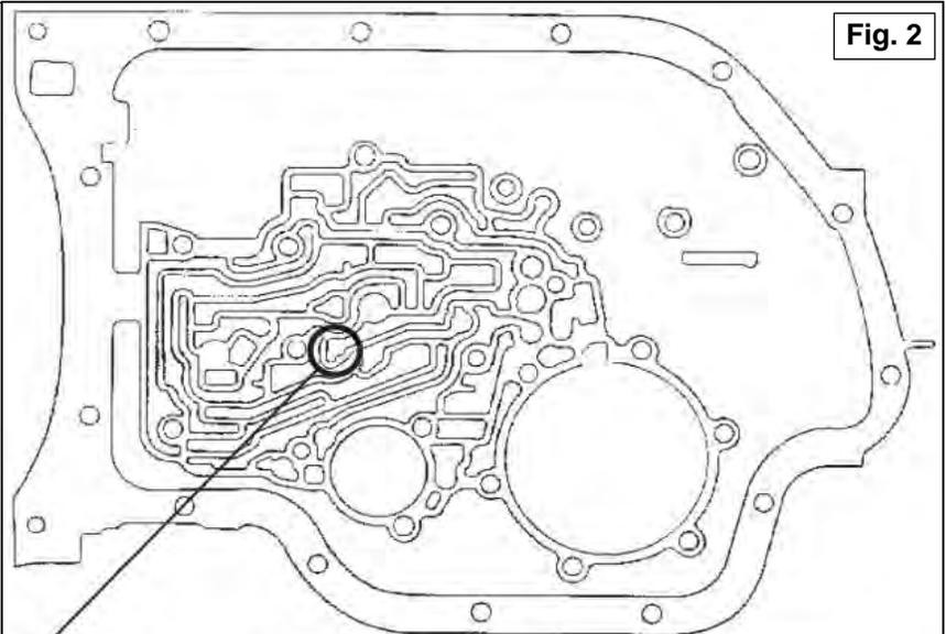
The 1987 and earlier TH-400 has no checkball in this location and must use Shift Improver Kit #20260. If you have a checkball in this location, this kit (#20261) is the correct one.
