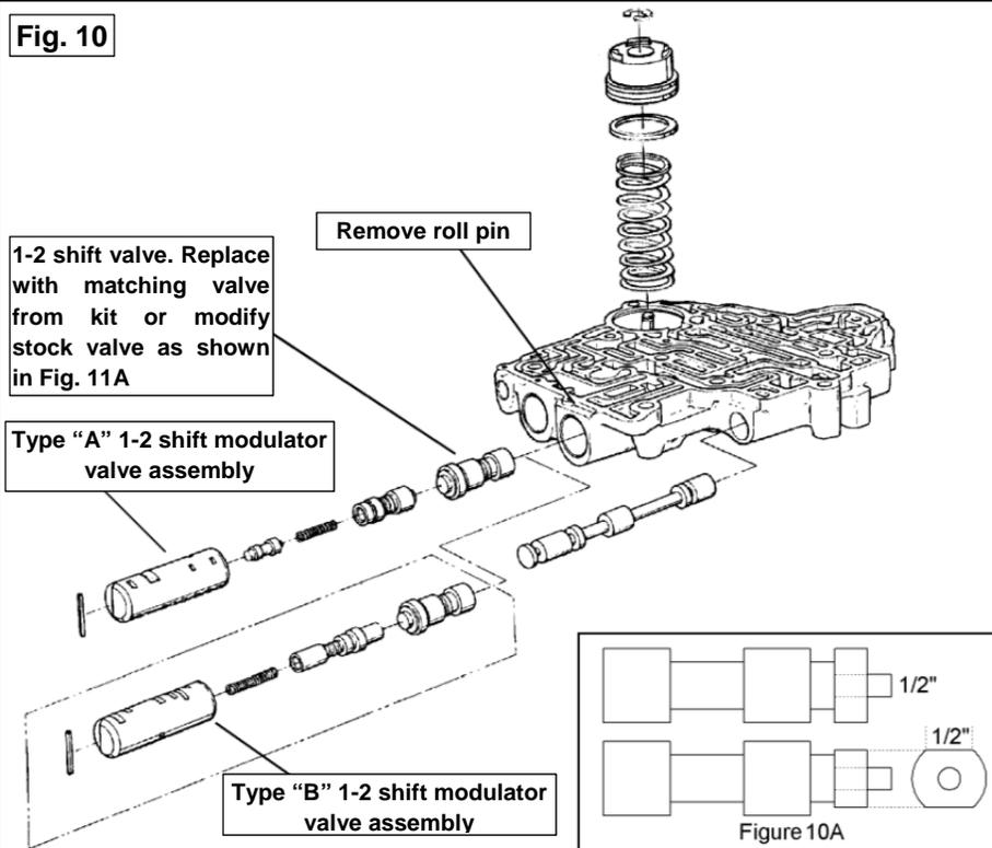
**Modification to stock valve:** Grind (2) 1/2" wide flats onto the land nearest the 1-2 spring (See Fig. 10A). Install the 1-2 shift valve into the bore with the smallest diameter pointing out (See Fig. 10). Reinstall the 1-2 shift modulator valve assembly as removed and replace the roll pin. Using a small screwdriver check to make sure the 1-2 shift valve slides back and forth freely.
