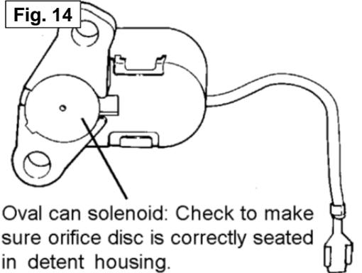
Oval can solenoid: Check to make sure orifice disk is correctly seated in detent housing.
