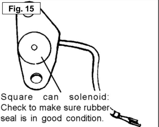
Square can solenoid: Check to make sure rubber seal is in good condition.
