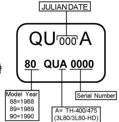
If the I.D. tag is unreadable or missing you will have to remove the oil pan and valve body from the transmission to determine if your transmission has an early or late style case (See Fig. 2). This kit will work correctly in all 1965-1987 TH-400 transmissions.
