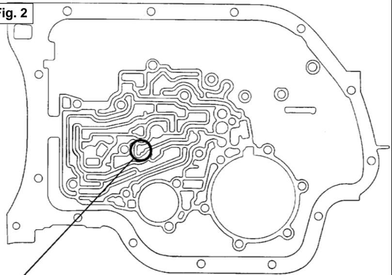
Make sure there is **no** checkball in this location. If 1988 and later TH-400 will have a checkball in this location in which this kit (#20228) will not work.
