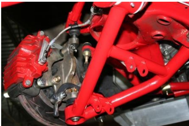
Figure 1: Lower A arm installed with Spindle
