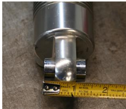
Figure 2: Measure the Bearing Sleeve Width
