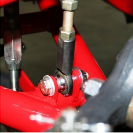
Figure 7: installed sway bar end link
