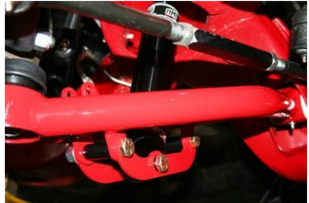
Figure 5: Installed Coil over. The black spacer will stick out of the front plate slightly.
