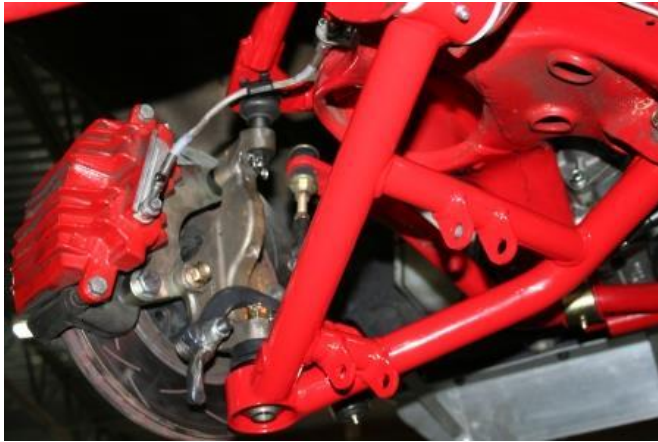
Figure 1: Lower A arm installed with Spindle
