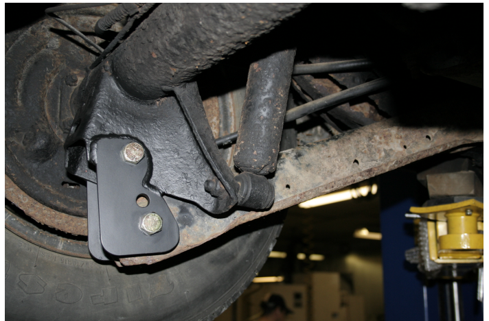
Image 2- Driver Side installed and welded
