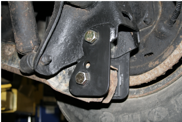
Image 1- Passenger side brackets installed and welded
