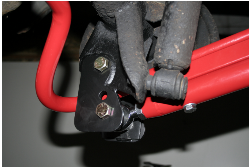
Image 3- Shows installation completed and brackets painted after welding. Shows item installed with item # 3612
