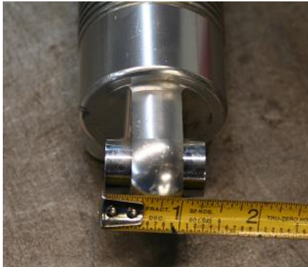
Figure 3: Measure the Bearing Sleeve Width
