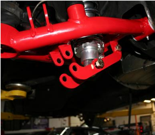
Figure 5: Attach Lower A-Arm Shock Mounts To the Shock
