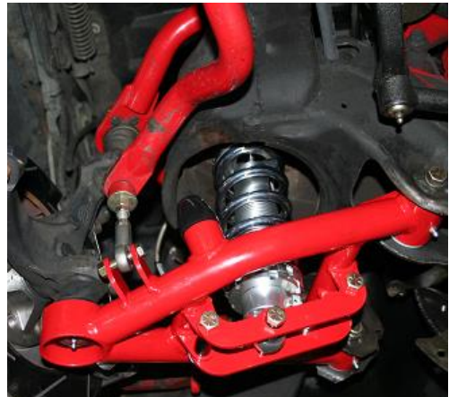
Figure 6: Install Final Shock Mount Bolt.
