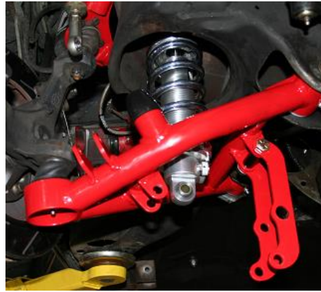
Figure 4: Install Shock To The Upper Mount. Adjuster Knobs toward Car Center
