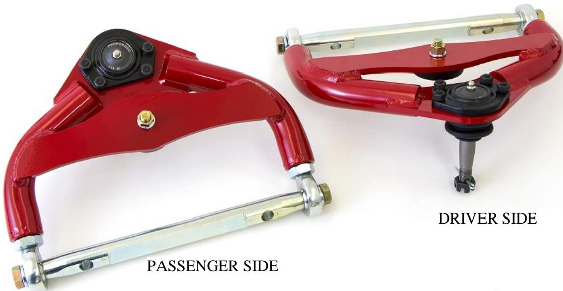
(Ball Joint to be ahead of centerline of cross-shaft)
