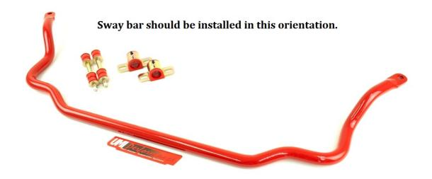
The photo above shows proper installation of the UMI 3035. Please do not install upside down as tie rod clearance trouble will occur. The UMI 3035 is shipped with endlinks intended to work with a majority of cars, reasonable ride heights and both standard and tall spindle heights (including tall ball joints or tall spindles). Excessive raising or lowering or use with other manufacturers products may require the purchase of shorter or longer endlinks.
