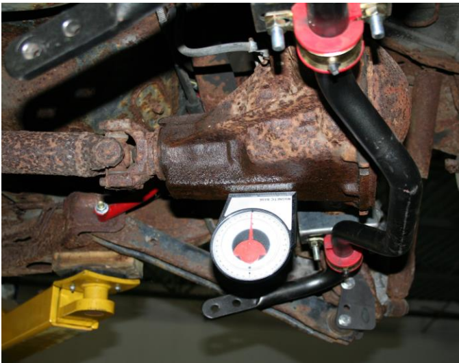
IMAGE #1: (Measure & Record Yoke Angle)
