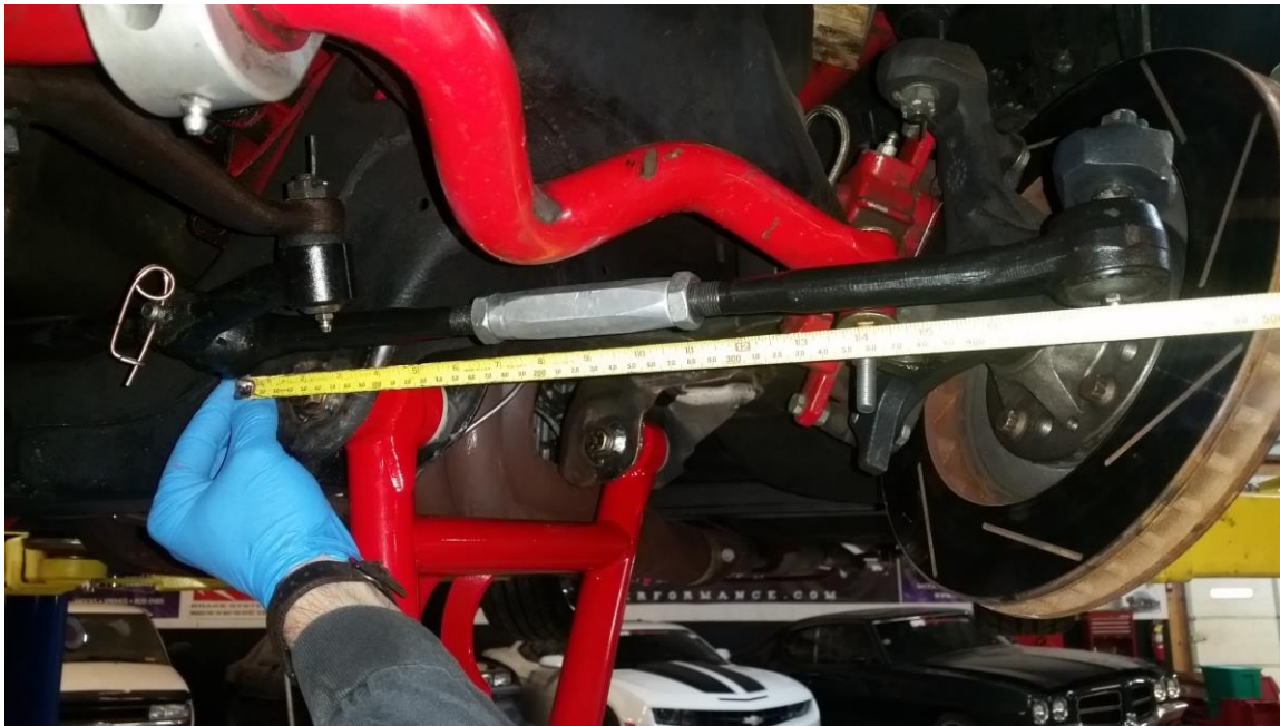
Figure 1: Measure initial tie-rod length
