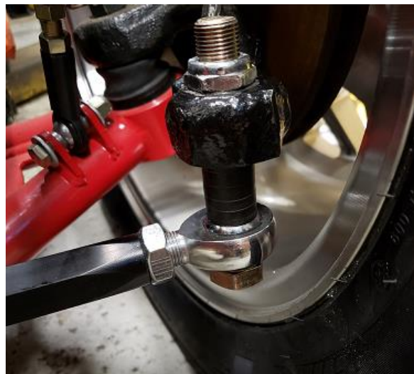
Figure 3: Bolt assembled with spacers
