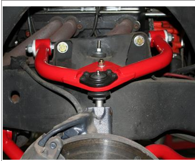
Installation Complete: Ball Joint offset Rearward
