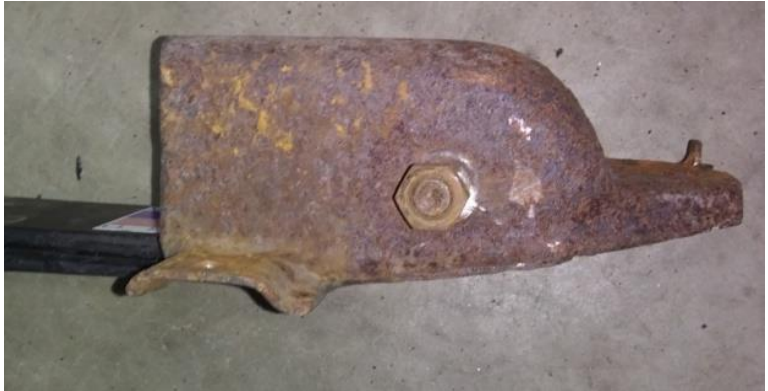
Front mount installed on spring
